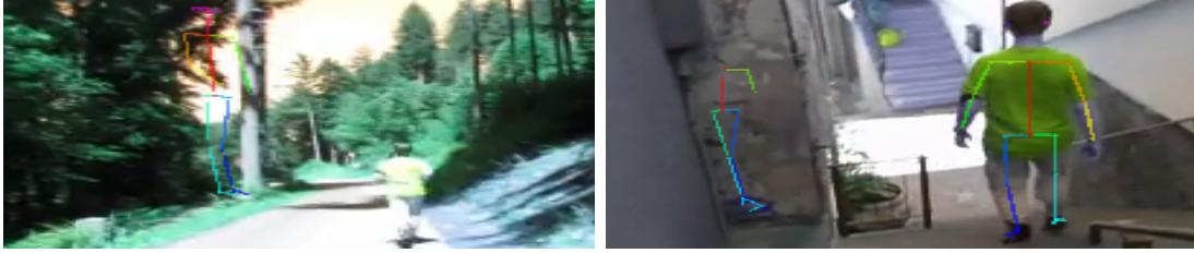
Figure 5.8: Typical fail cases of OpenPose in our video data preprocessing, with downscaled video frames, background objects are wrongly recognized as human.
