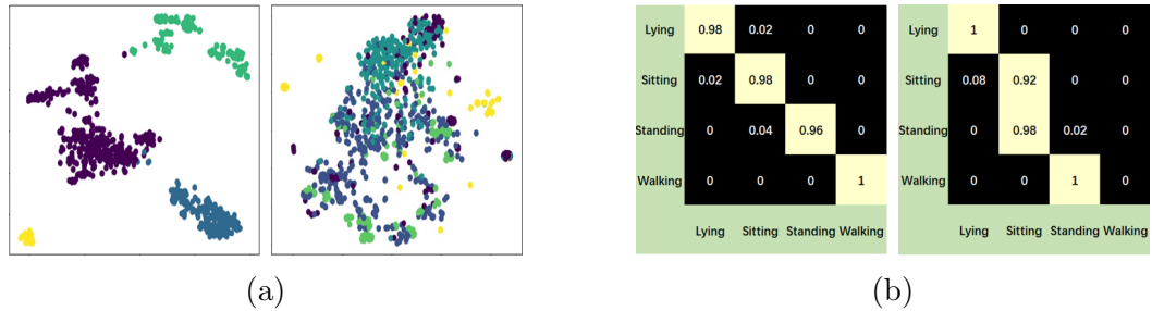
Figure 3.1: Typical data variance problem caused by subject difference and device diversity. (a) depicts the impact of subject difference, where different colors in the t-SNE plots denote different activities. (b) shows the impact of device diversity. Left confusion matrix shows predictions on device seen to the model while right confusion matrix from a new unseen one. The prediction on unseen device’s data is totally confused except for the ‘lying’ activity.
