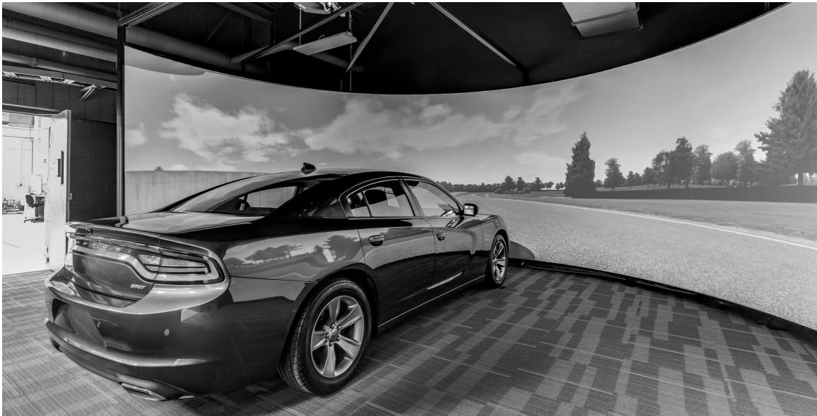
Figure 2.4: Static driving simulator at the MARCdrive lab.
