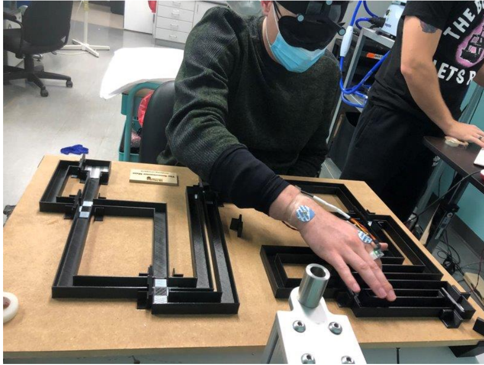
Figure 9: Maze Training- Image of participant performing a maze training trial. Notice that participant is seated and blindfolded, forcing them to rely on tactile information from the intersections to navigate through the maze.
