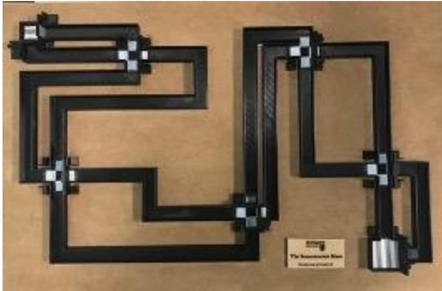
Figure 7: Tactile Discrimination Maze- Overhead view of the paths on the maze board. Black pathways are the maze surface explored by the finger. Start/End zones indicated by white/grey stripes.
