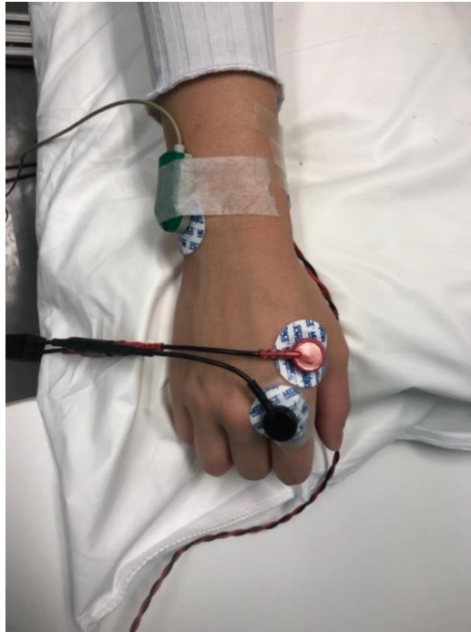
Figure 4: EMG Electrode Setup- Organization of electrodes used to record muscle activity during the study. Active electrode over the muscle belly of the right first dorsal interosseus (red), reference electrode over the right knuckle (black), and ground electrode on the styloid process of the ulna (green).
