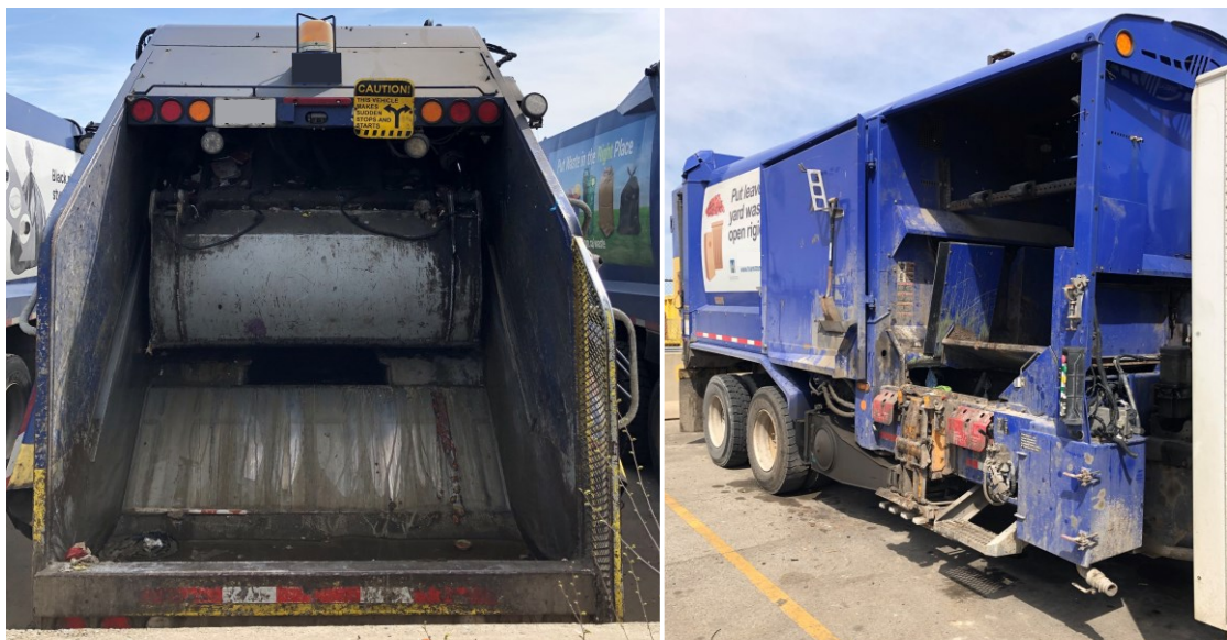
Figure 5.2: The rear-loading compaction chamber (left). The split side-loading compaction chambers (right).
