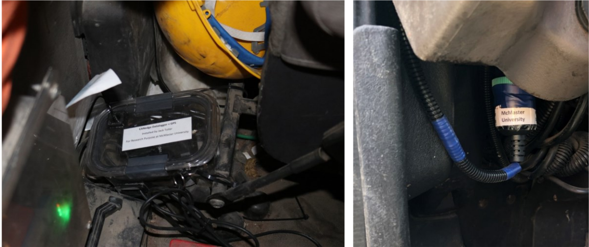
Figure 4.6: The data logger installed into the split side-loading rural/urban truck. Left: The data logger unit was placed behind the driver's seat. Right: The J1939 connection is by the steering wheel column.
