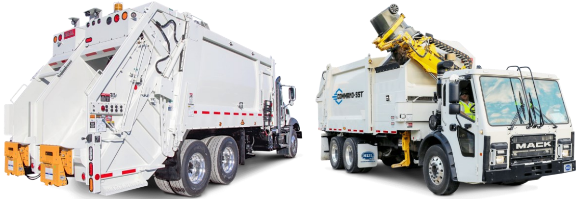
Figure 2.8: Split rear-loader refuse truck (left). Heil automated side-loading refuse truck (right) [1].
