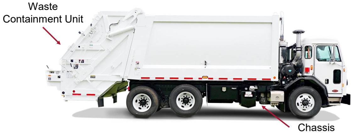
Figure 2.3: The Anatomy of a refuse truck, including the chassis and waste collection unit [1].
