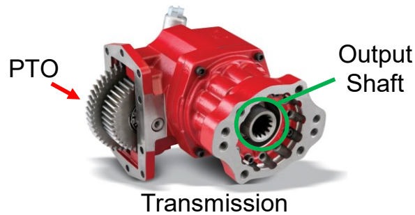
Figure 2.5: A schematic showing the power take-off connection on a multi-speed automatic transmission
