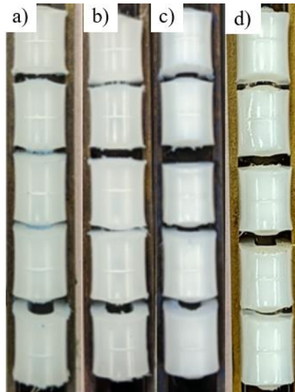
Figure 4.4. Washed and dried polyethylene test specimens immersed in a 0.10 wt% Bromocresol Green solution, a) HD8660.29 (552 hours), b) LL8460.29 (552 hours), c) LA080 (552 hours), d) HD9830.02 (168 hours)
