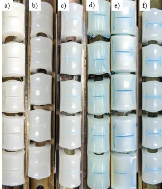
Figure 4.3. Coloration of washed and dried LA080 specimens after 48 h immersed in the solution containing a) 10% IGEPAL CO-630 without Bromocresol Green, or 10% IGEPAL CO-630 with Bromocresol Green at concentrations of b) 0.0005 wt%, c) 0.005 wt%, d) 0.01 wt%, e) 0.025wt%, f) 0.05 wt%.
