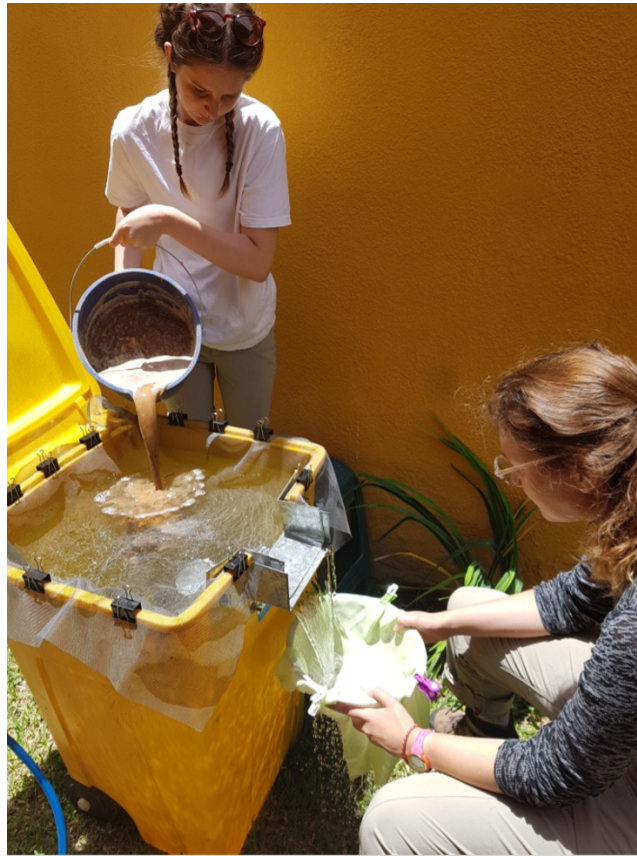
Figure 4.1: Modified SMAP flotation machine in use by S. Watson and H. Dine (Photo by S. Morell-Hart) (Morell-Hart et al. 2018:149)
