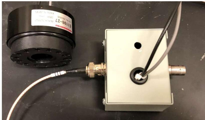
*Figure 2.8: Interface for the setup without preamp*
