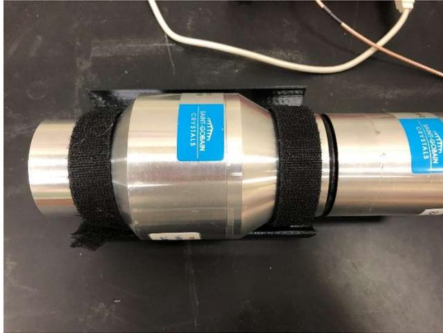
*Figure 1.1: Picture of the LaBr<sub>3</sub>(Ce) used for experiment*
