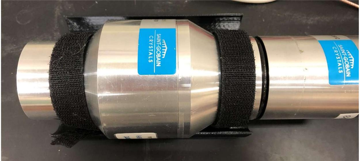
*Figure 2.5: LaBr<sub>3</sub>(Ce) detector used for measurements (With Preamp unit attached)*
