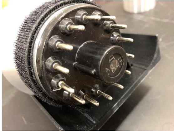
*Figure 2.6: Port for preamp unit connection*
