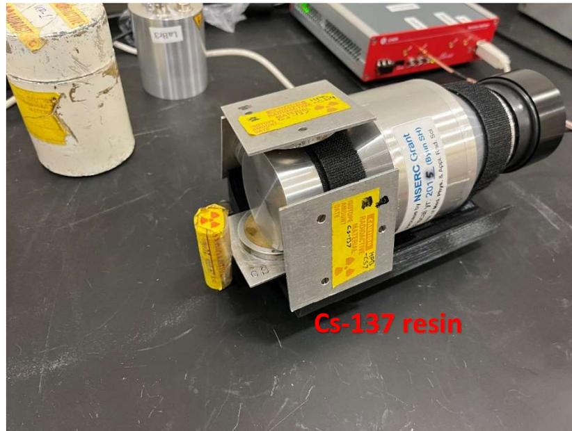
*Figure 4.2: Source arrangement for resin source measurements*
