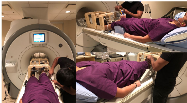
FIGURE 6.8: Pre-scan set up with participant in position for right leg plantar flexion paradigm on built ergometer pedal housing and wooden participant bed.
