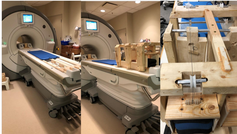
FIGURE 6.7: Built ergometer pedal housing design and wooden participant bed. Left image shows wood participant bed interfacing with the MRI table (cover removed), middle image shows ergometer housing and wood bed interfacing, and right image shows the pulley mechanics in the plantar-flexion orientation
