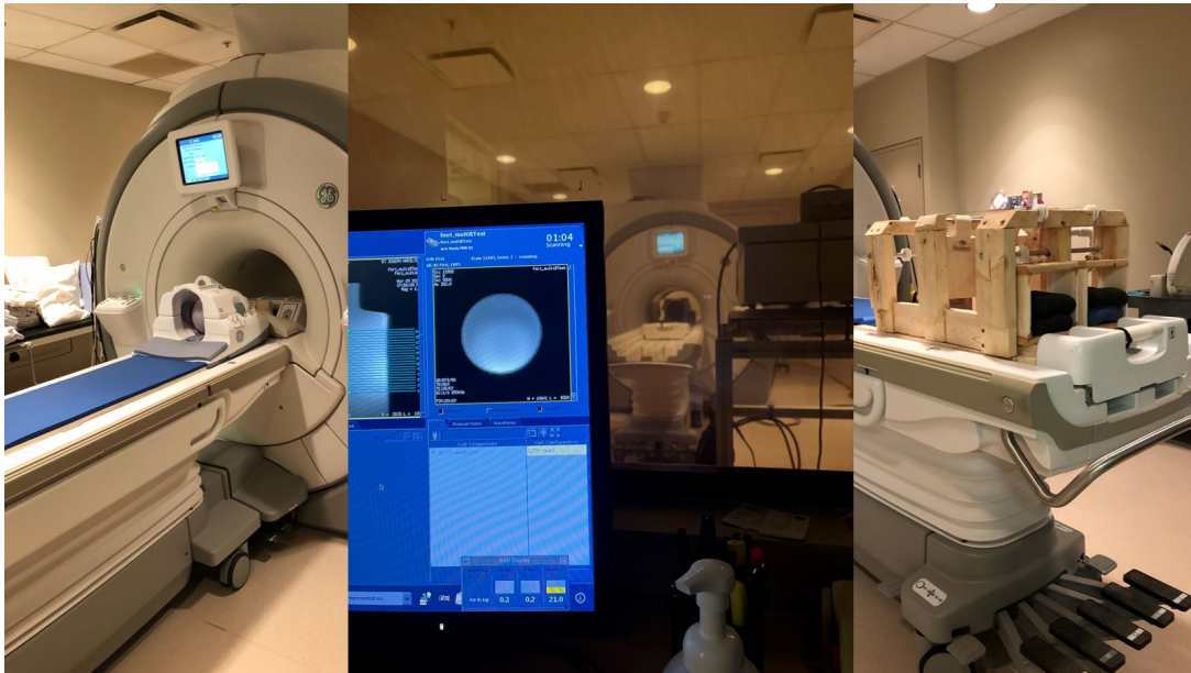
FIGURE 6.9: QA Set-up. Left image with the HNS coil containing the 3T cylindrical phantom. Middle image showing the central slices of the phantom used for analysis. Right image showing the foot pedals positioned at the foot of the scanner bed for a fMRI scan.
