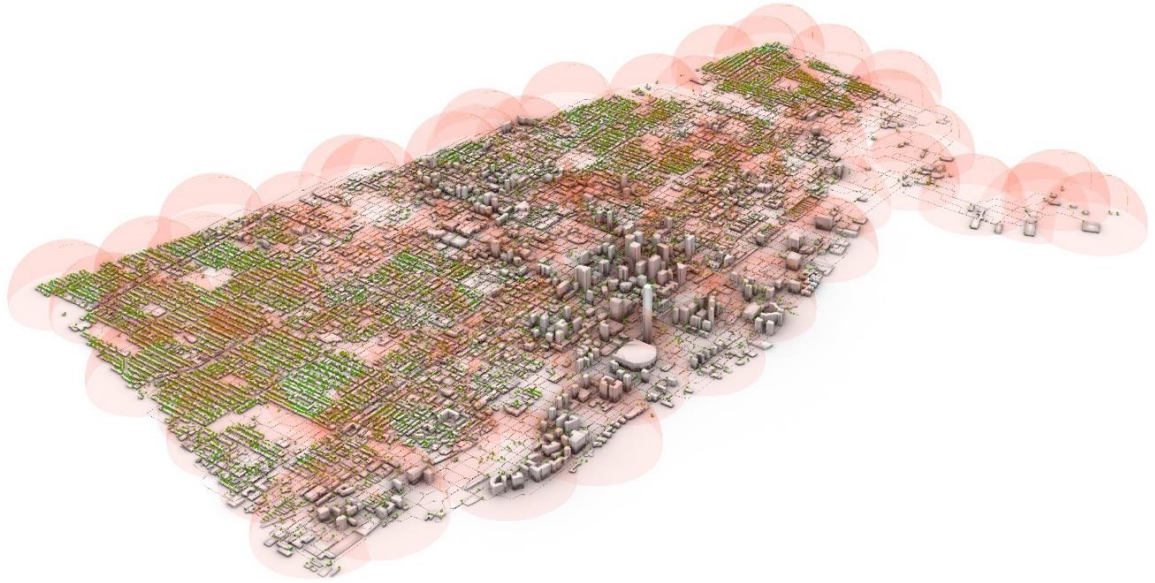
Figure 6-7 Optimized charging coverage map for the case study of Toronto.
