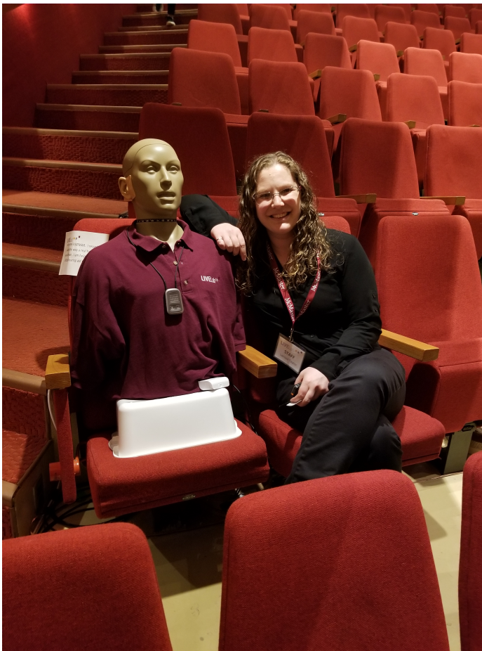
Figure 6.3: KEMAR manikin used for recording and feed setup, with researcher Larissa Taylor.
