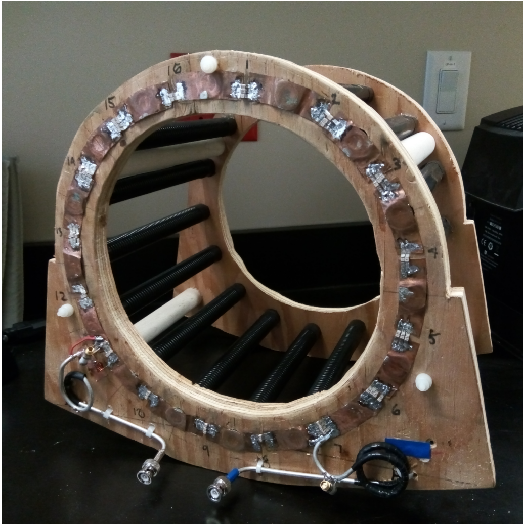
Figure 4.1: A single-channel, single-tune, transmit and receive quadrature bird-cage RF coil. This coil is tuned to 33.8 MHz, the Larmor frequency for ^{23}\text{Na} at 3 T. Its inner diameter is designed to contain an imaging field of view (FOV) of 240 mm, typically large enough for an adult human head. This is the coil which was used in the experiments detailed in the rest of this manuscript.
