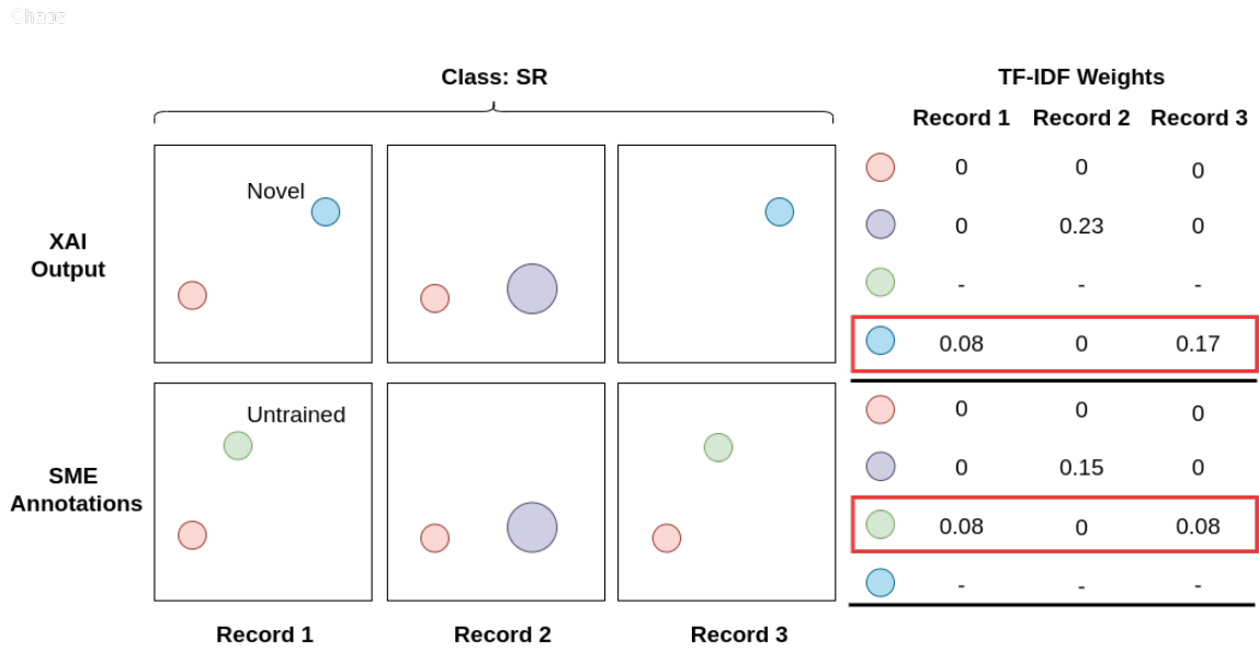
Figure 2.9: Visualization of TF-IDF used to determine the significance of features identified by an XAI output and SME annotations for a given record. Each record is an ECG test sample, coloured circles represent features, blue and green features are novel and overlooked features respectively.
