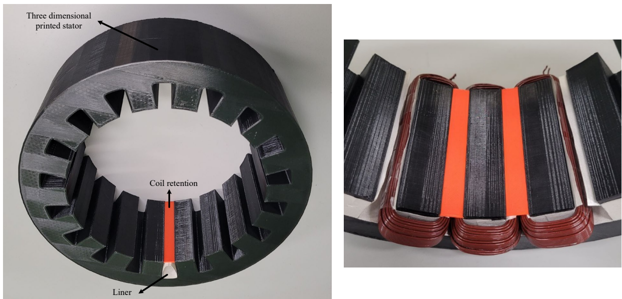
Fig. 6-11. 3D printed stator with coil retention for validation of strength and tolerance.
