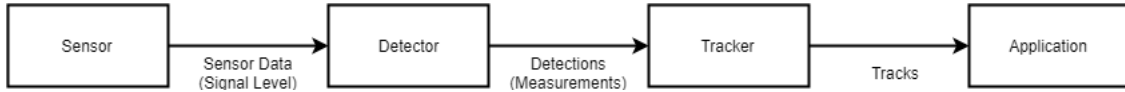
Figure 1.1: A simple tracking framework using real sensor data. Note that the ground truth is not known when capturing real data.
