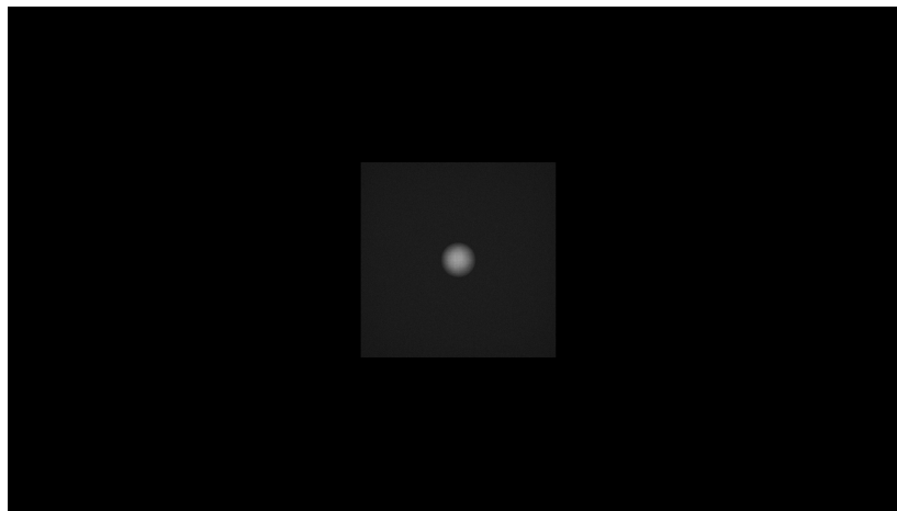
Figure 3.7: A simulated camera image for the scenario described in section 3.2.4.2. The spherical target is visible in the center of the image, seen through the transmissive pane. The transmissive pane is also partially visible because of its material's diffuse component.
