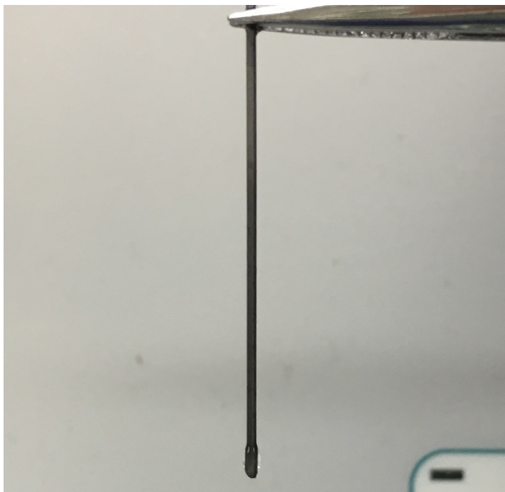
Figure A.2: Picture of a modified pencil lead electrode wetted and holding water. Unmodified pencil lead would not wet and hold water.
