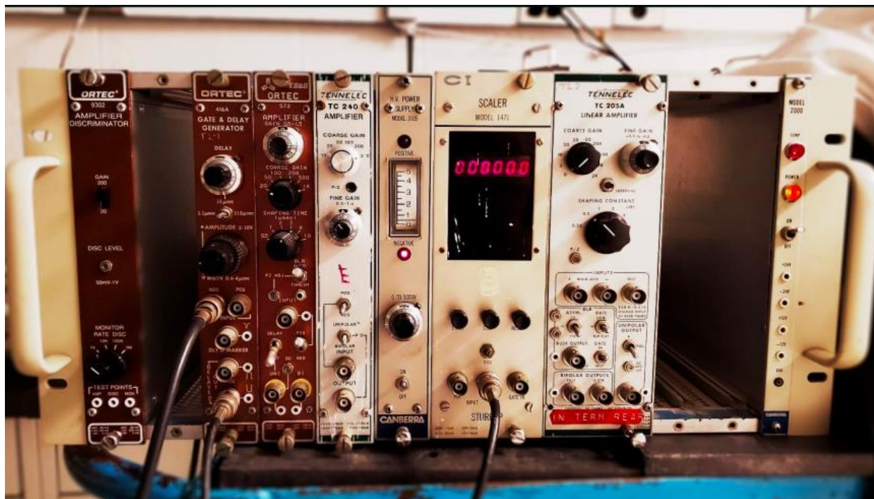
Supplementary Figure 1.2 Nuclear Instrumentation Module (NIM) of Photon Counter. The panels used for operating the photon counter is seen here. The power to the NIM is found on the right side. The power was turned on and voltage on the HV Power panel was turned on and dialed to -800V for 30 minutes before use, to allow for the apparatus to “warm up”. The Stop, Start and Reset buttons on the Scaler panel were used to respectively start, stop and reset photon counts during detection. All other dials and setting remained the same, as set up by previous students in the laboratory. This image was taken by and courtesy of Andrej Rusin (2021).
