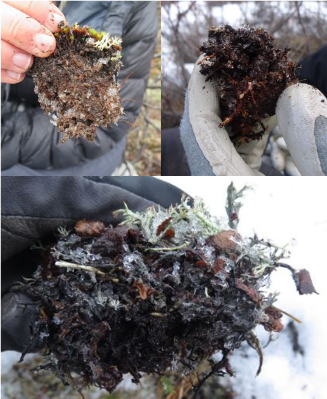
Figure 3.3a-c: Examples of frozen soils with ice impeding pore space at the sampled sites.
