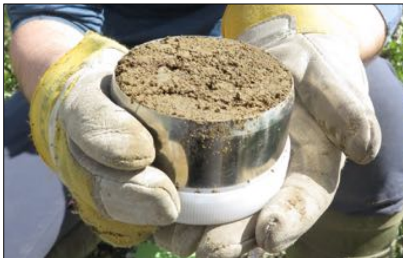
Figure 3.5: UMS HYPROP 250 mL soil ring sample in field.
