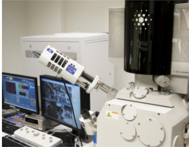
Figure 2.1: The FEI Magellan 400, a high-resolution SEM.
