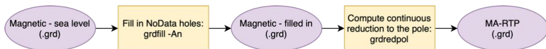
Figure 11: Procedure to fill NoData holes and compute the RTP anomaly from the MA data set.
