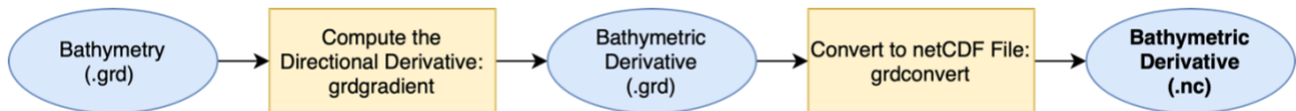
Figure 9: Compute the directional derivative of the bathymetry data and convert to netCDF file.
