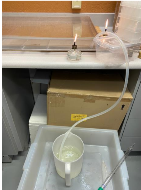
Figure 8: Overnight MEGA-plate bleaching and drainage set-up. The bleach drainage set-up consists of using a serological pipette and plastic tubing to create a pressure difference that allows bleach to drain in a bucket.
