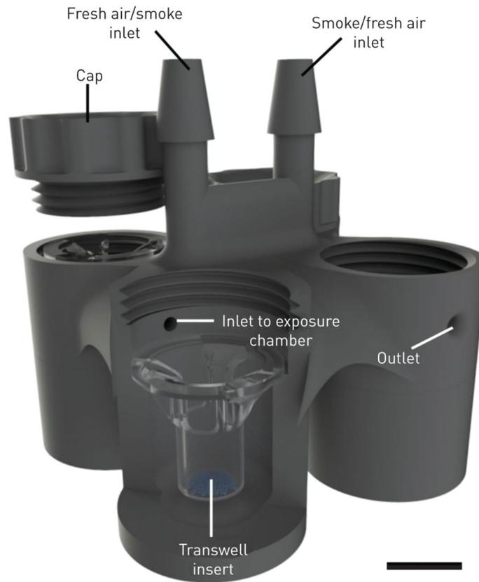
**Figure 1. Three-dimensional schematic view of the *in vitro* exposure system.** As shown, air or exposure (*e.g.* smoke) delivered to the inlet is equally distributed across the four exposure chambers which house the Transwell inserts. Circulated air or exposure (*e.g.* smoke) exits passively through the outlet in each exposure chamber. Scale bar = 1 cm.
