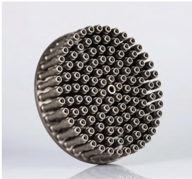
FIGURE 1.3: Injector head of a rocket engine printed from IN718 superalloy using EOS laser powder bed fusion technology [23].
