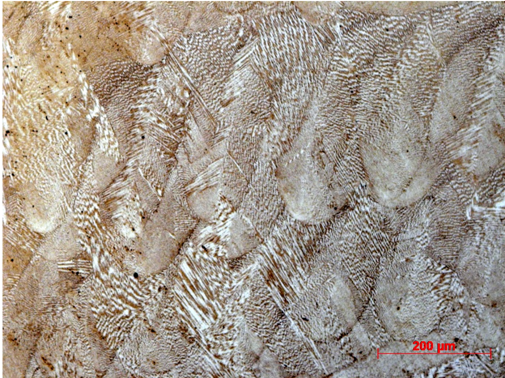
FIGURE 4.42: Optical micrograph showing the microstructure of L-PBF IN625 printed with set 4 processing parameters.
