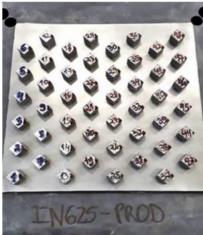
FIGURE 4.23: 48 IN625 cubes ( 10 \times 10 \times 10 \text{ mm}^3 ) printed with P = 400 \text{ W} , v = 700, 900, 1100, 1300 \text{ mm/s} , t = 60, 90, 120, 150 \mu\text{m} , and overlap = 10, 30, 50%.
