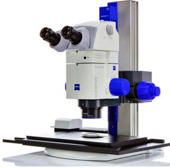
FIGURE 3.6: Stereoscope ZEISS SteREO Discovery.V8 used for analysis the top views of the tracks.
