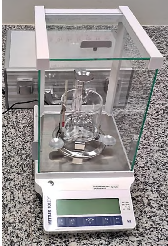
FIGURE 3.9: Digital electronic balance used for measuring the density.
