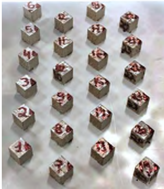
FIGURE 4.36: 24 IN625 cubes printed with P = 400 W. (i) Cubes 1–6 printed with v = 1300 mm/s, t = 60 \mu\text{m} , 30% overlap, and h = 84 \mu\text{m} . (ii) Cubes 7–12 printed with v = 1200 mm/s, t = 90 \mu\text{m} , 50% overlap, and h = 56 \mu\text{m} . (iii) Cubes 13–18 printed with v = 700 mm/s, t = 120 \mu\text{m} , 50% overlap, and h = 83 \mu\text{m} . (iv) Cubes 19–24 printed with v = 700 mm/s, t = 150 \mu\text{m} , 50% overlap, and h = 77 \mu\text{m} .
