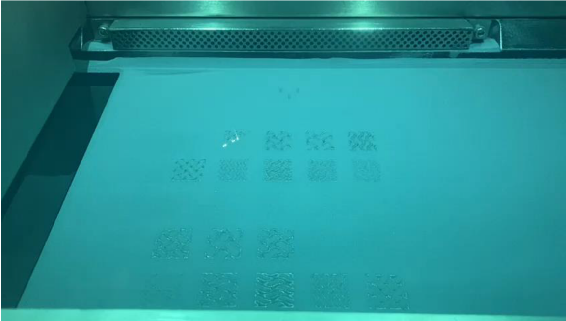
Figure 3.18: Samples getting printed using LPBF in EOS M280
