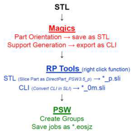
Figure B.1: Process to create file for printing
