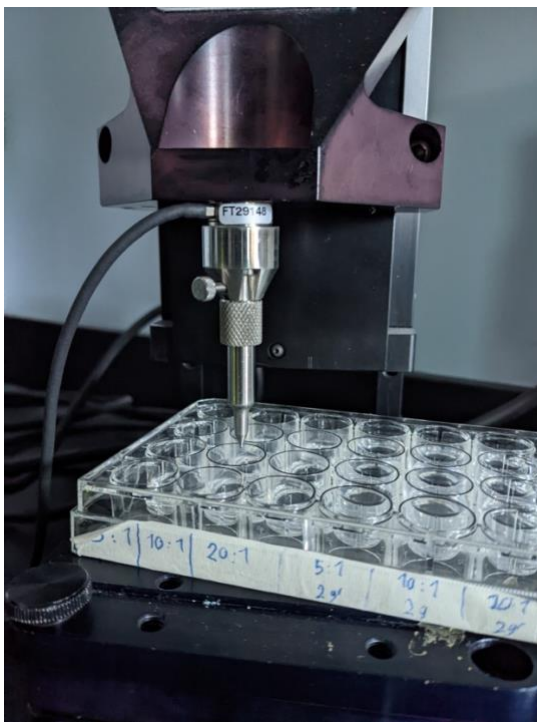
Figure S2: Picture of Biomomentum mechanical testing set-up with spherical indenter attachment
