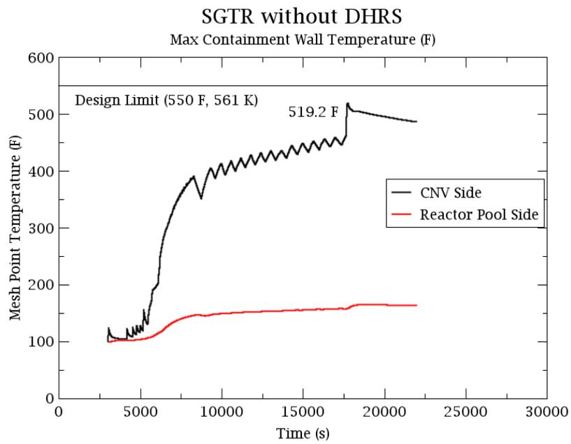
Figure 35: Containment wall temperature in a transient SGTR without DHRS event.
