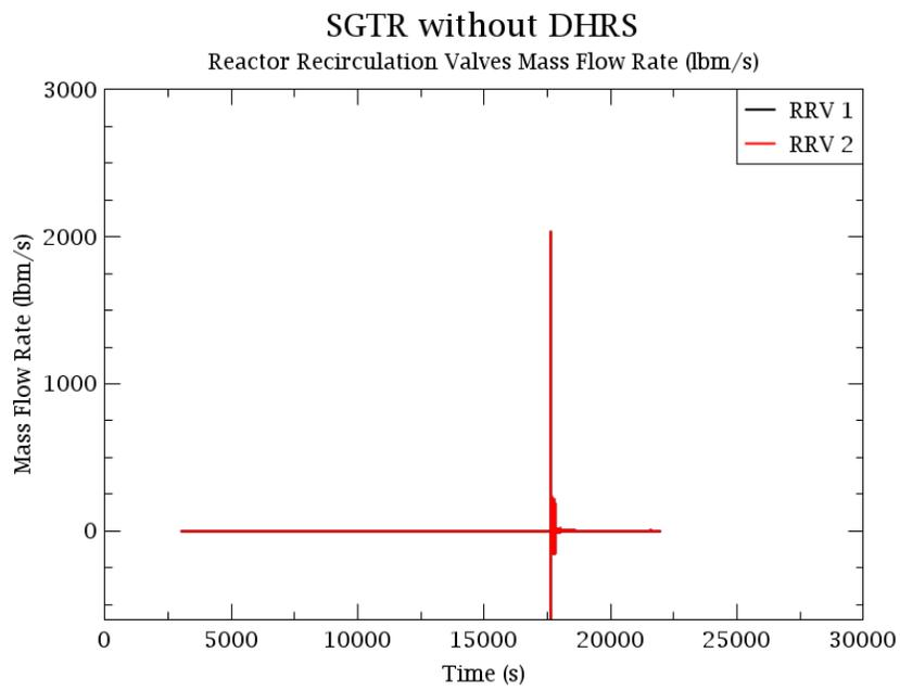
Figure 36: Reactor recirculation valve flow rates in a transient SGTR without DHRS event.
