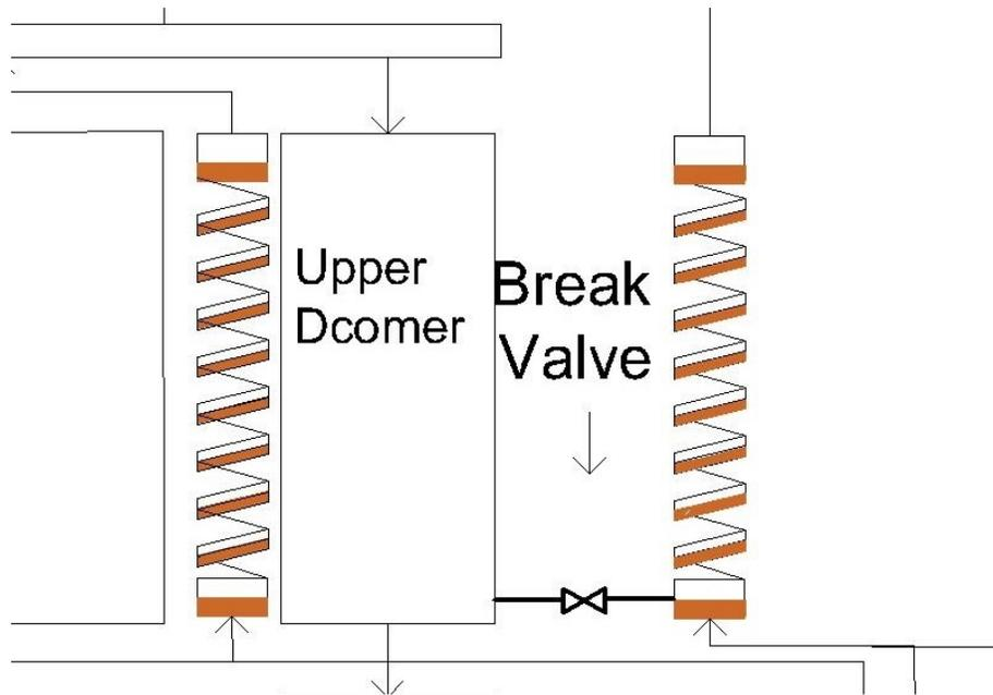
Figure 16: Changed break valve RELAP model for SGTR event
