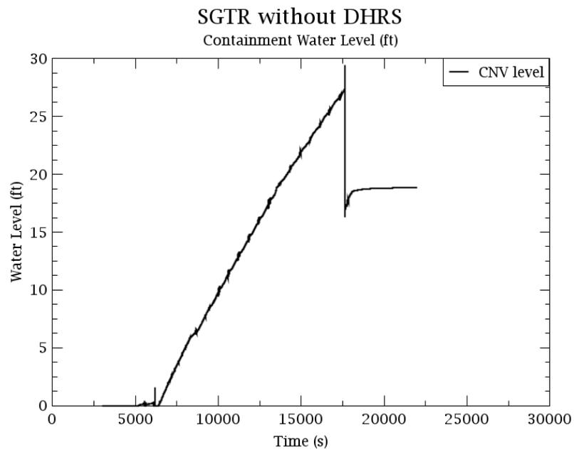
Figure 33: CNV level in a transient SGTR without DHRS event.
