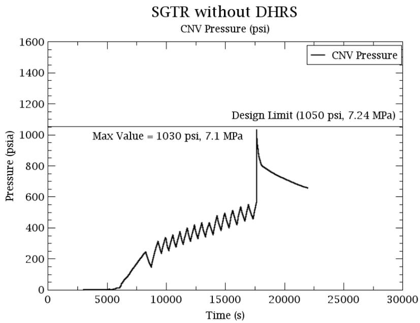
Figure 32: Containment pressure in a transient SGTR without DHRS event.
