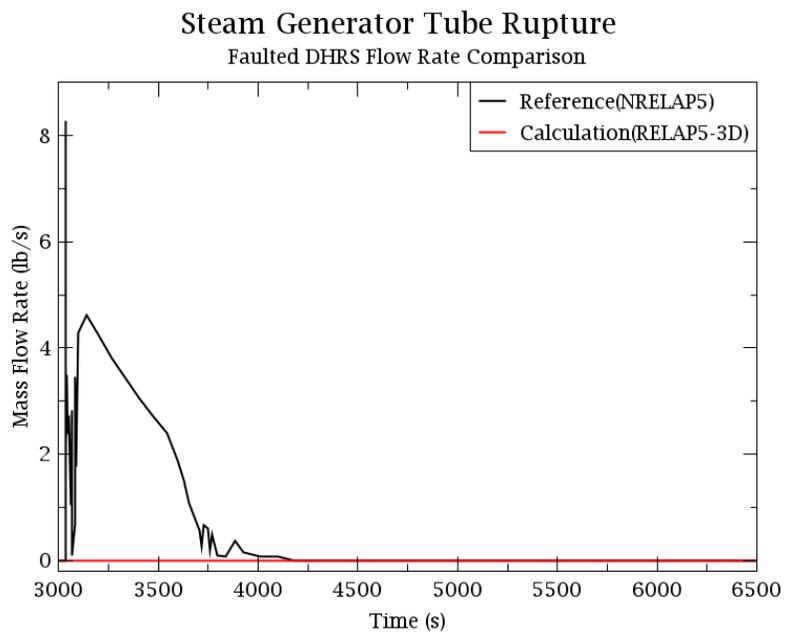
Figure 24: Faulted DHRS1 mass flow rate in a transient SGTR event.
