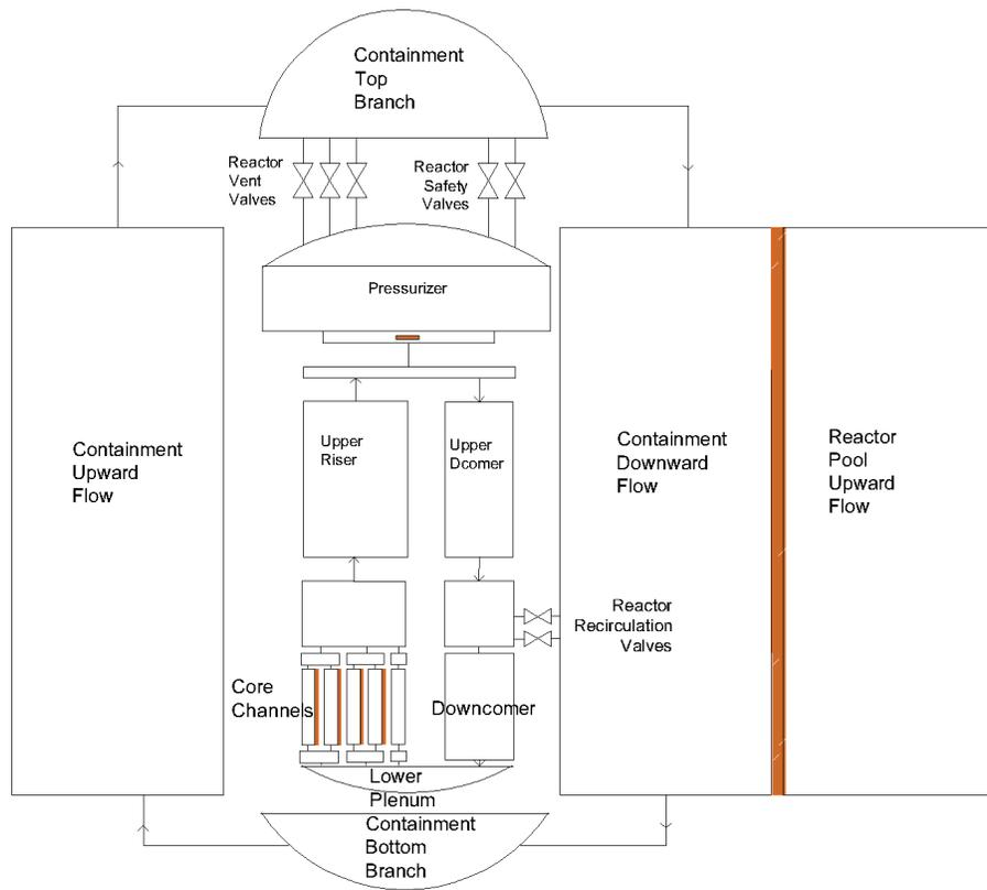
Figure 12: Containment vessel and ECCS modeling.
