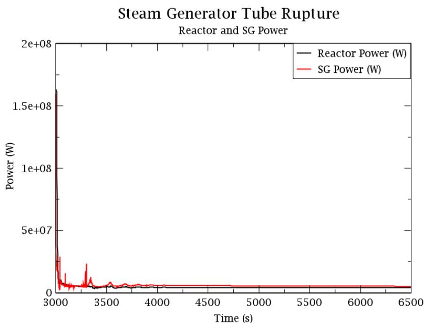
Figure 20: Reactor and steam generator power in a transient SGTR event.
