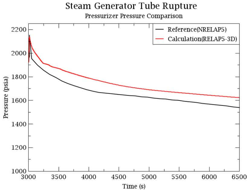
Figure 21: Pressurizer pressure in a transient SGTR event.
