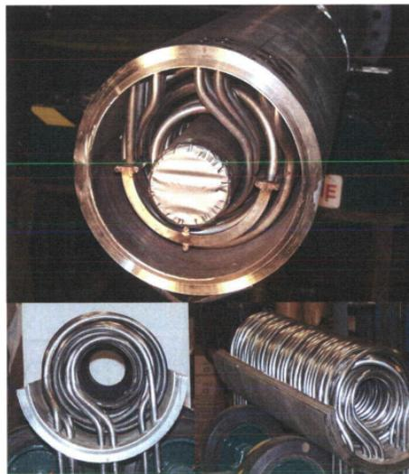
Figure 5: Helical Coil Steam Generators in TF-2 NIST Test Reactor
