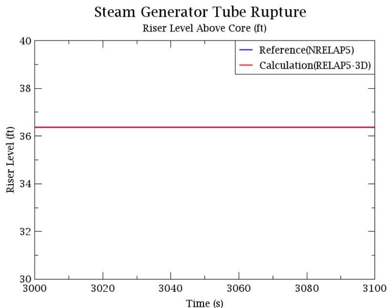
Figure 26: Riser water level in a transient SGTR event.
