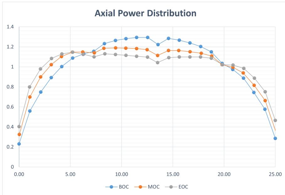
Figure 10: Axial power profile in the NuScale power module [2].
