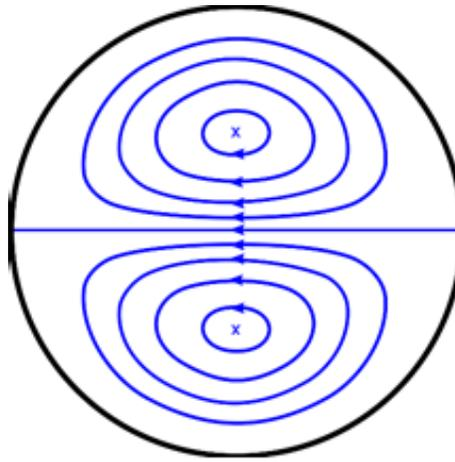
Figure 6: Schematic of a pair of Dean vortices that form in curved pipes.
