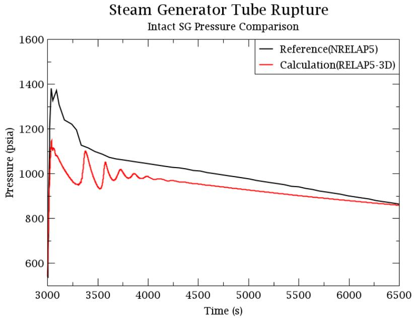
Figure 23: Intact SG pressure in a transient SGTR event.
