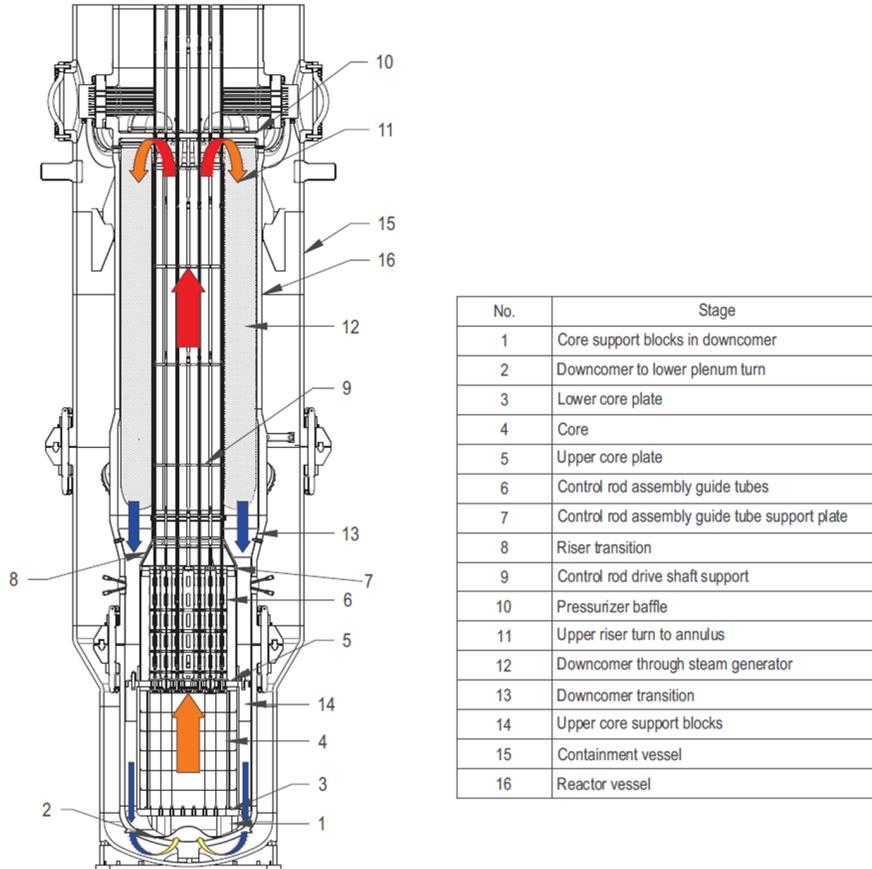
Figure 2: The NuScale Reactor Coolant System.[3]
