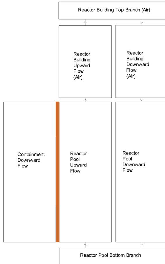
Figure 13: Reactor pool modeling.
