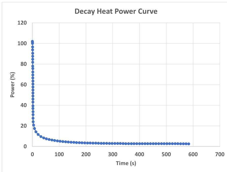
Figure 17: Decay heat power after reactor shutdown
