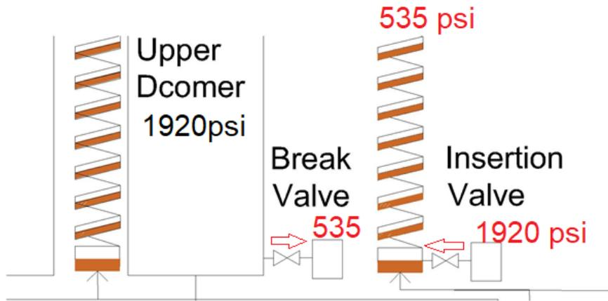
Figure 15: Break Valve RELAP Model for SGTR Event
