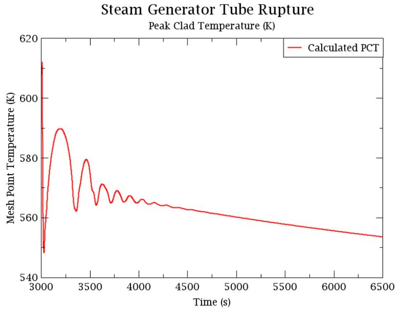
Figure 27: Peak clad temperature in hot channel in a transient SGTR event.
