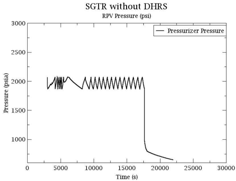
Figure 31: Pressurizer pressure in transient SGTR without DHRS event.
