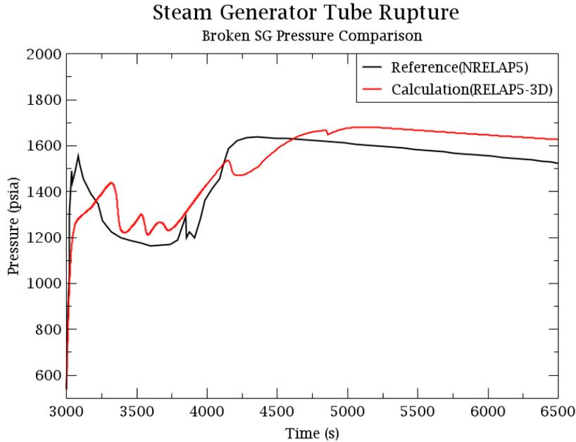
Figure 22: Faulted SG pressure in a transient SGTR event.
