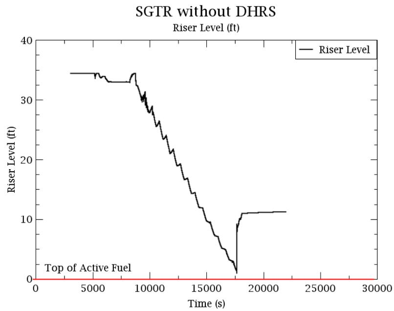
Figure 34: Riser level in a transient SGTR without DHRS event.
