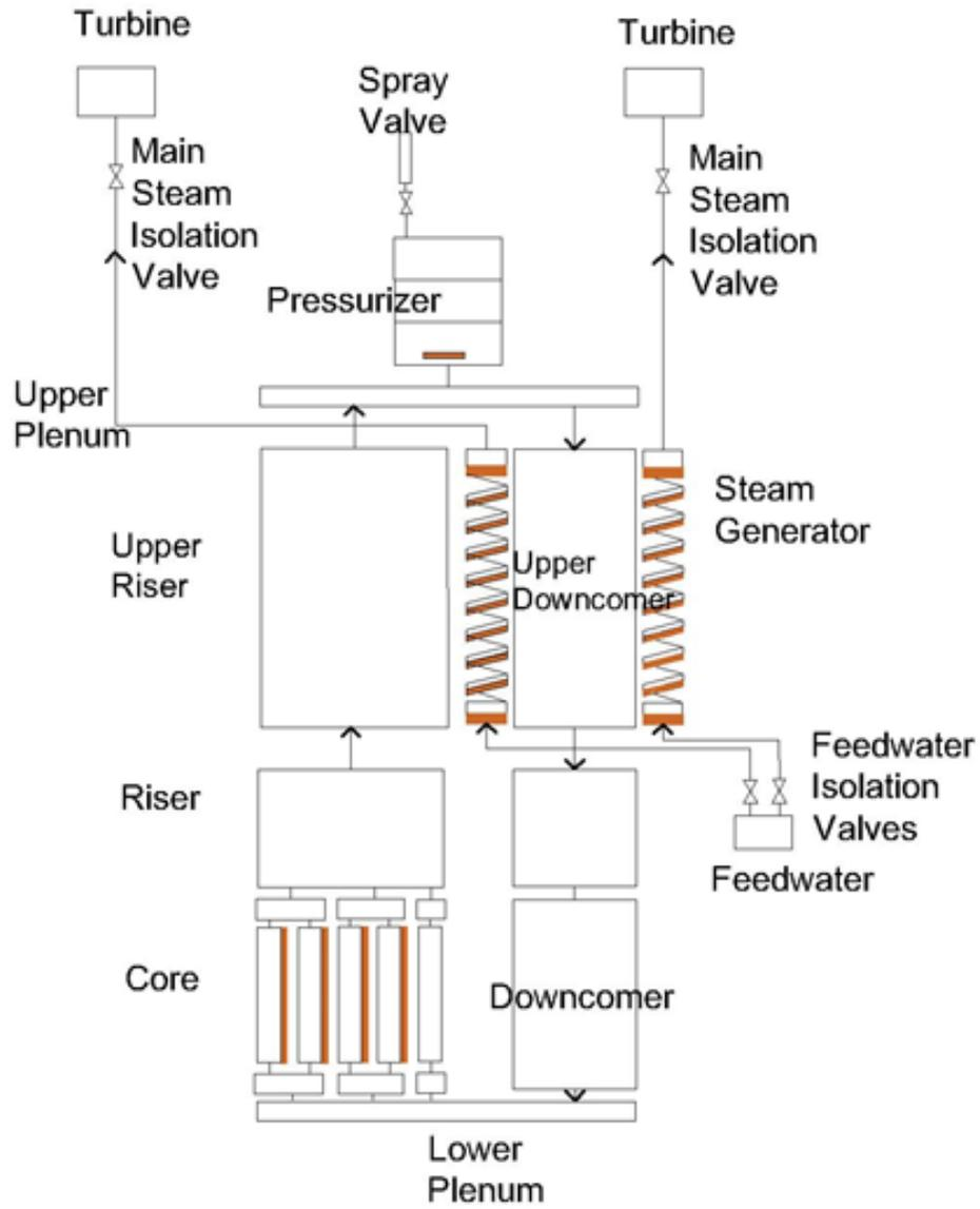
Figure 8: Improved nodalization for natural circulation stability.
