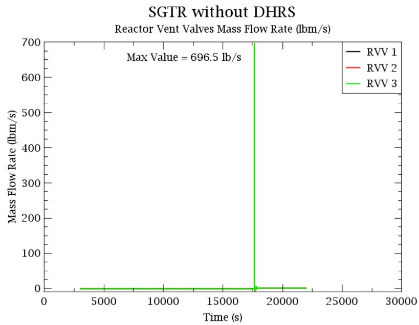
Figure 37: Reactor vent valve flow rates in a transient SGTR without DHRS event.
