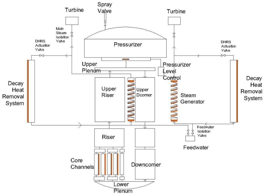
Figure 9: Nodalization with Decay Heat Removal System Added
