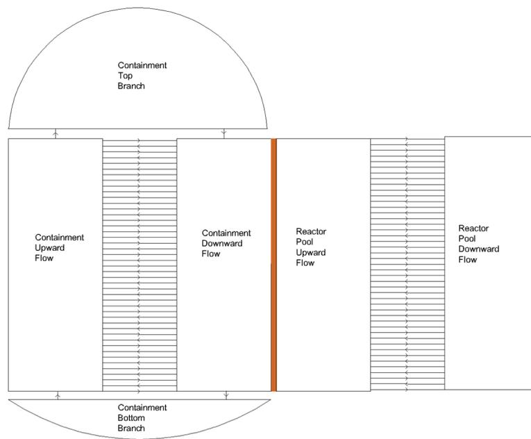
Figure 14: Containment and reactor pool multiple junction connections.
