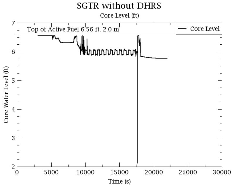
Figure 30: Core water level in a transient SGTR without DHRS event.
