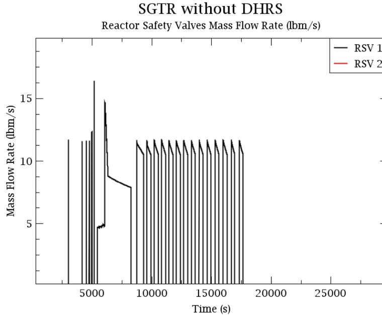
Figure 29: Reactor safety valve flow rates in a transient SGTR without DHRS event.
