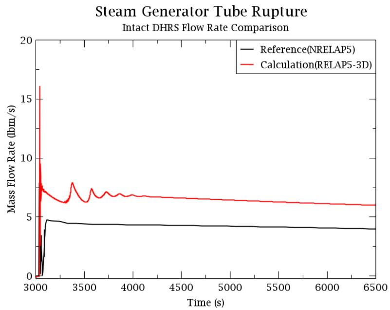
Figure 25: Intact DHRS mass flow rate in transient SGTR event.
