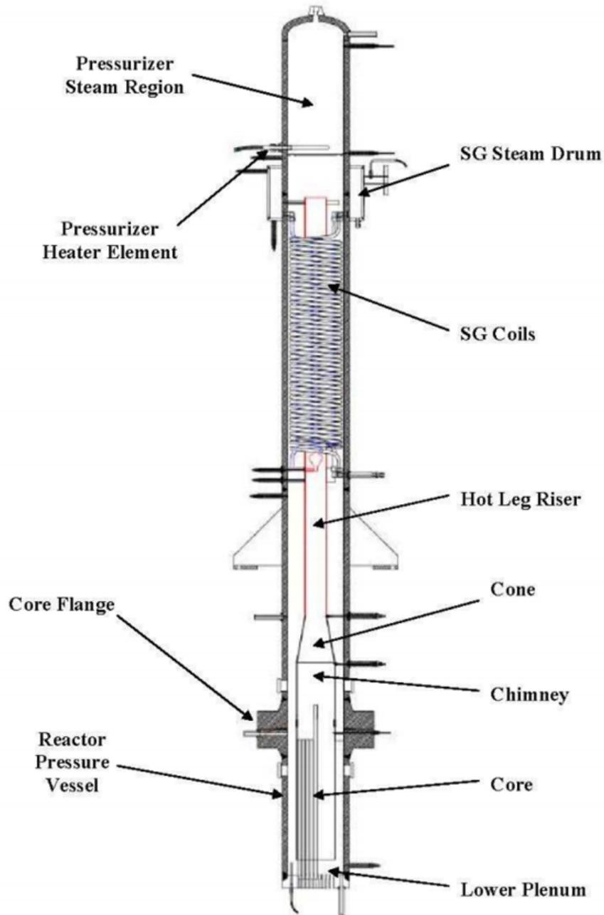
Figure 1: MASLWR Test Facility Schematic at Oregon State University [6]
