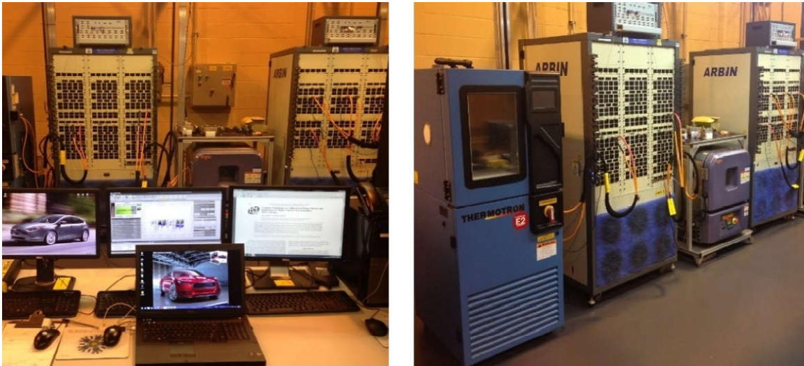
Figure 3.6: Experimental setup including cyclers, environmental chambers, and Data Acquisition systems [16].
