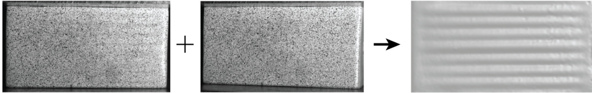
Figure 2.9 3D reconstruction of a compressed bearing surface using 3D-DIC
