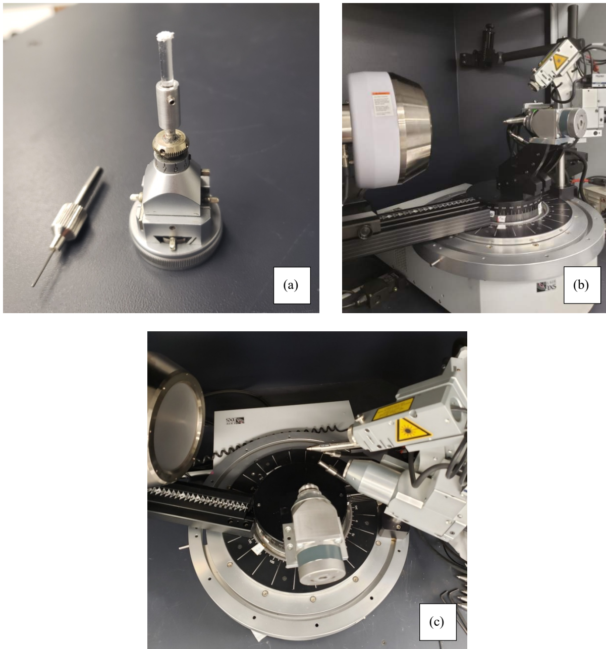
Figure 2.4. Images of (a) approximately 100 \mu\text{g} powdered precipitate mounted on the XRD sample mount which is then loaded into the (b)/(c) Bruker D8 DISCOVER diffractometer equipped with a Bruker Vantex600 area detector, and a \text{CuK}\alpha sealed tube source for characterization.
