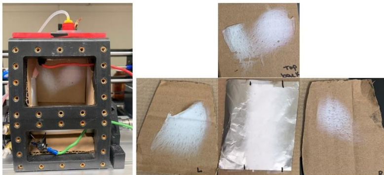
Figure D3. Example of off-target fiber deposition (severe splatter).
