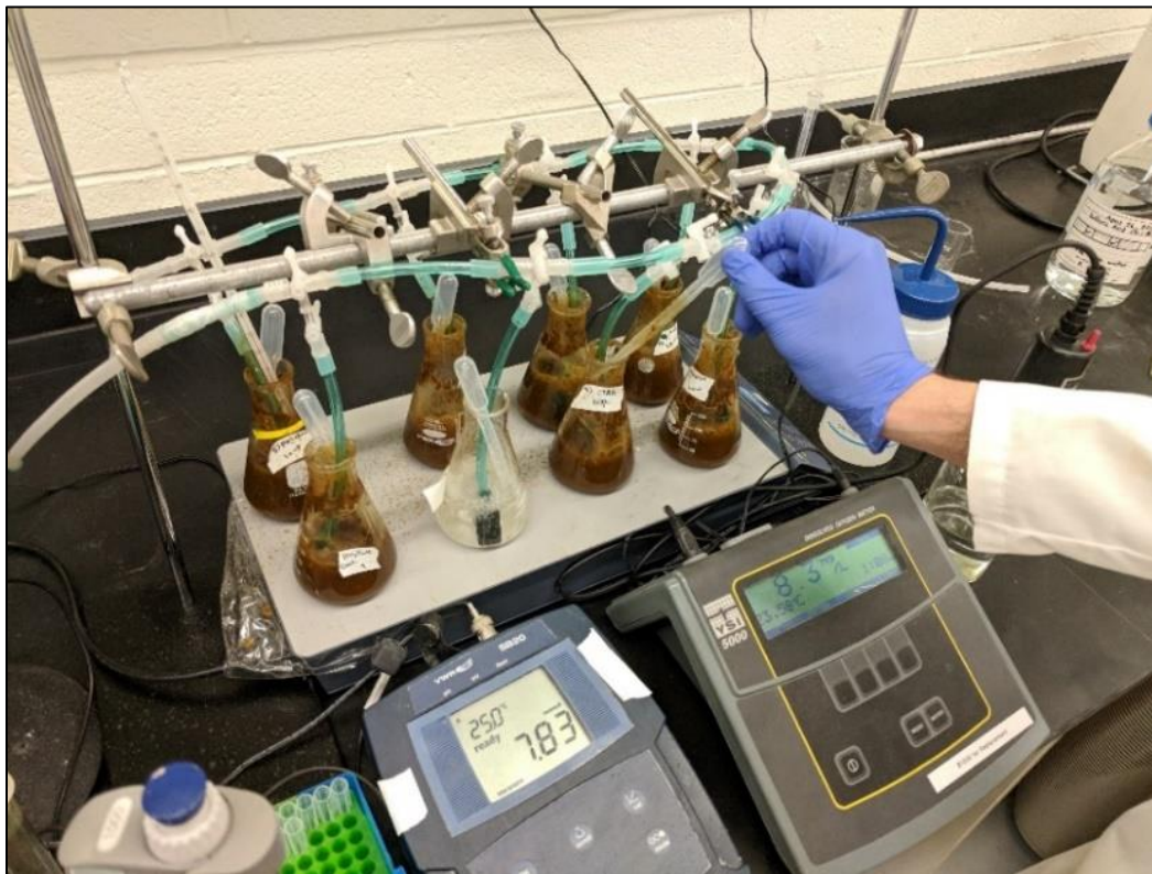
Figure B2. SNR experimental setup: pH meter, dissolved oxygen meter, seven 100 mL Erlenmeyer flasks containing return activated sludge, mineral medium, COD medium, and the corresponding WW sample. This figure shows a user sampling an SNR batch reactor for measurement of nitrite-N and nitrate-N concentrations. The clear Erlenmeyer flask was not used in this study; typically, this flask would represent the SNR control and would look identical in color to the other flasks (Milli-Q water exposure instead of a WW sample).
