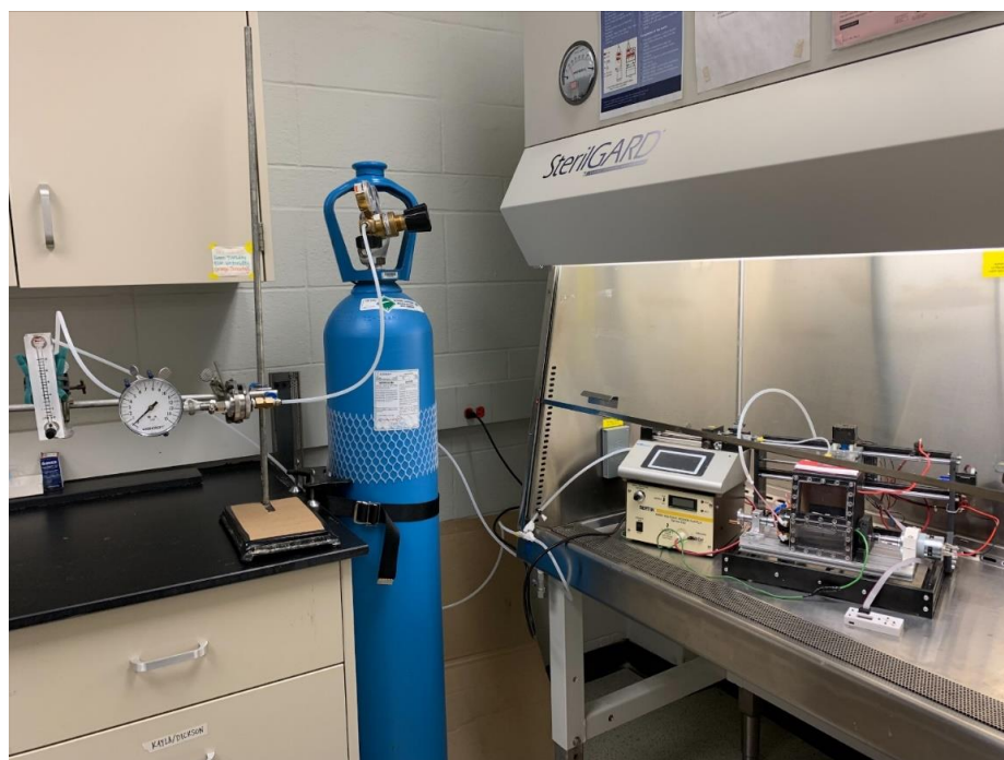
Figure D2. Electrospinning system in a Baker SterilGARD III Advance ® SG403A Class II, Type A2 Biological Safety Cabinet (The Baker Company) with the nitrogen gas cylinder setup including a pressure gauge and a rotameter for controlling nitrogen gas flow rate into the E-Box.
