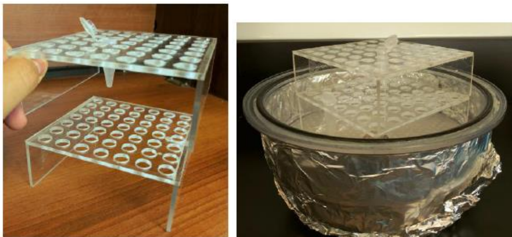
Figure A2. Left: two tube-holding racks (stackable). Right: Two tube-holding racks stacked and placed into an xL Bel-Art Vacuum Desiccator.
