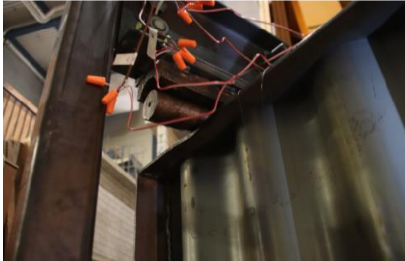
Figure 3-9: WTA610 Local Flange Failure
