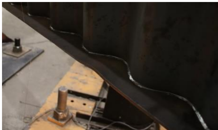
Figure A-19: Faint Local Flange Buckling of the Deformed WTA333/127x6 – 9
