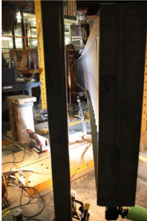
Figure A-8: End Profile of the Deformed WTA610/127x6
