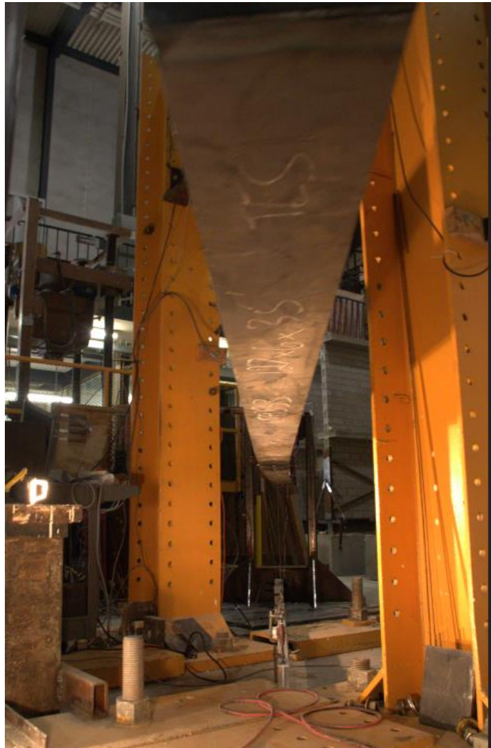
Figure A-3: Compression Flange of the Deformed WTA333/127x6 – 2
