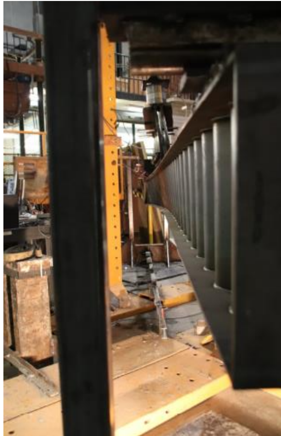
Figure A-18: End Profile of the Deformed WTA333/127x6 – 9
