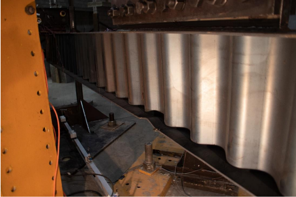
Figure A-2: Side Profile of the Deformed WTA333/127x6 – 1
