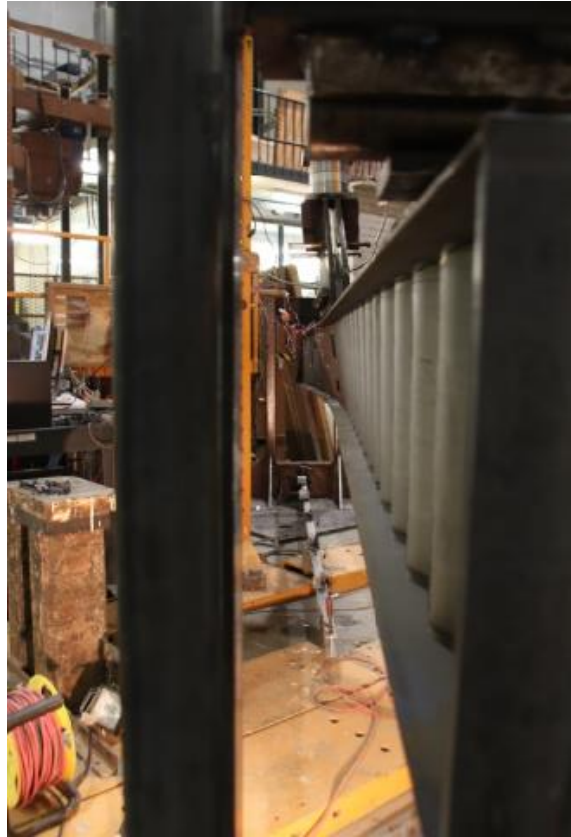
Figure A-14: End Profile of the Deformed WTC333/127x6
