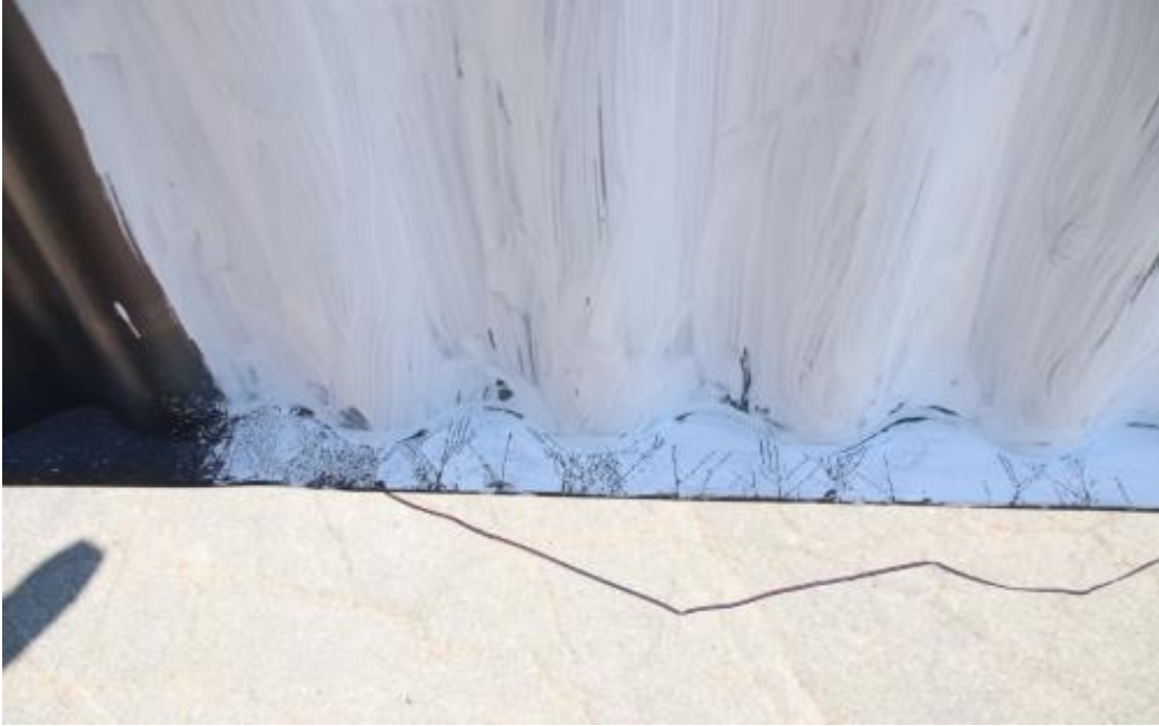
Figure A-11: Local Flange Buckling and Yielding of the Deformed WTA750/127x6
