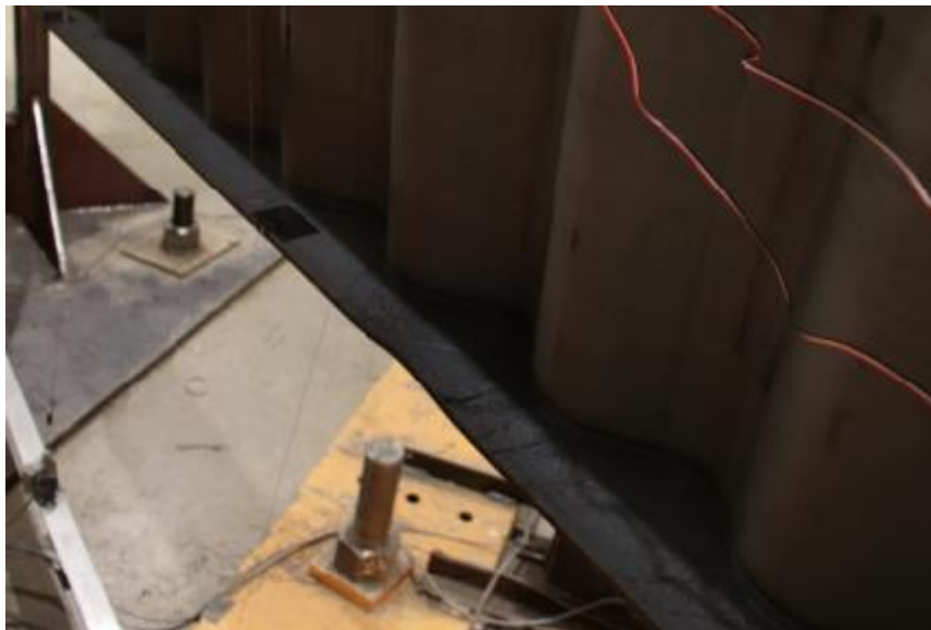
Figure A-15: Local Flange Buckling of the Deformed WTC333/127x6
