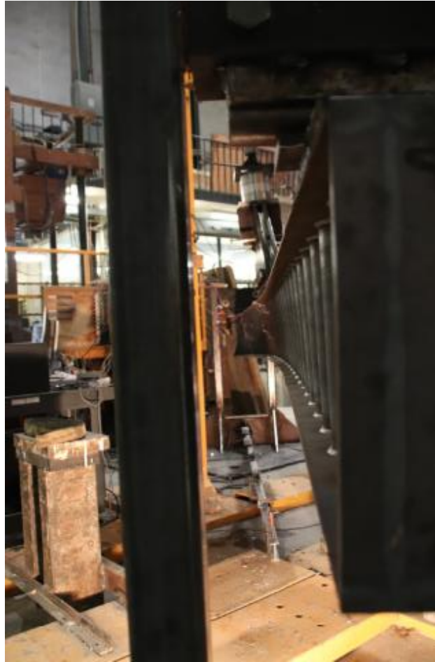
Figure A-16: End Profile of the Deformed WTF333/127x6
