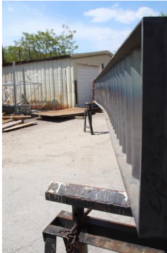
Figure A-5: End Profile of the Deformed WTA500/127x6
