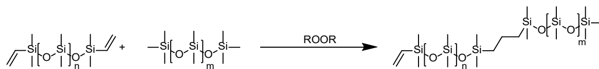
Figure 1.6: Peroxide-radical initiated vulcanization of a silicone elastomer at elevated temperatures. ROOR represents a peroxide initiator.
