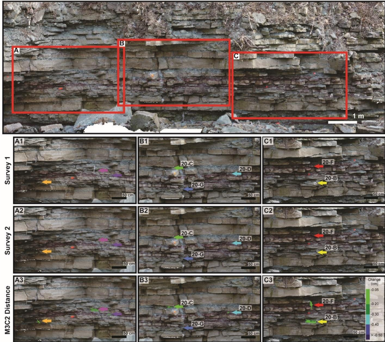
Figure 4.8: Top: Overview of the outcrop studied in 2020 showing the location of the three areas of sampling with images of areas of removed samples enlarged below. Survey 1 of the outcrop with all sample locations indicated by coloured arrows, see Figure 4.5 for sample close-up (A1; B1; C1); B) Survey 2 of the outcrop with the location of the samples indicated (A2; B2; C2). Sample 20-G (B3) did not register any change in the M3C2 point cloud; C) Results of the M3C2 algorithm showing the calculated change for the removed samples overlain on Survey 2 imagery (A3; B3; C3). Seven of the eight removed samples were identified using the algorithm, with Sample 20-G (B1-3) considered a false negative in this analysis.
