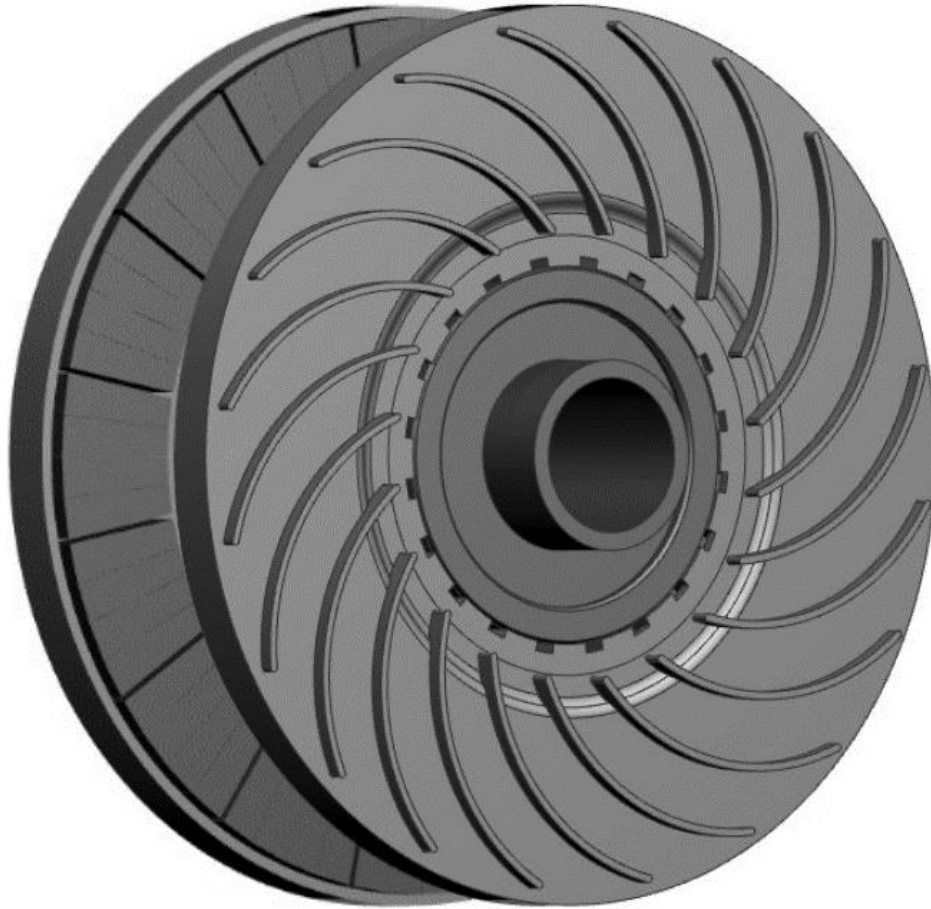
Fig. 4-25 R4 rotor design, rotor with backward curved fan blades.
