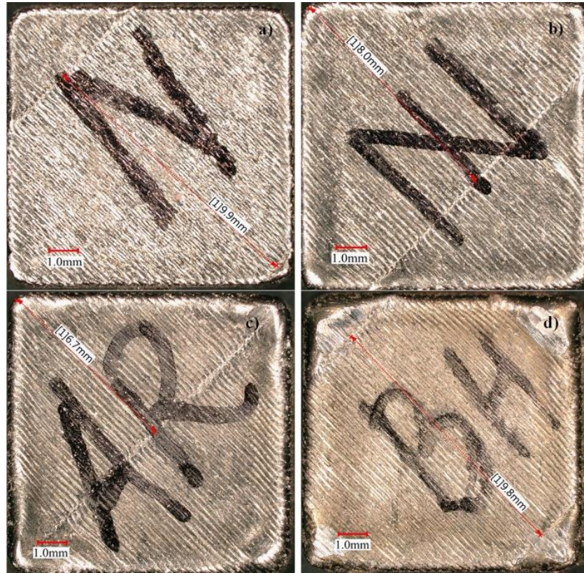
Figure 2-18 Variation of scan track length on the top surface for a scan speed of 550 mm/s and hatch spacing of 0.1 mm at a laser power of a) 140 W b) 170 W c) 220 W d) 270 W
