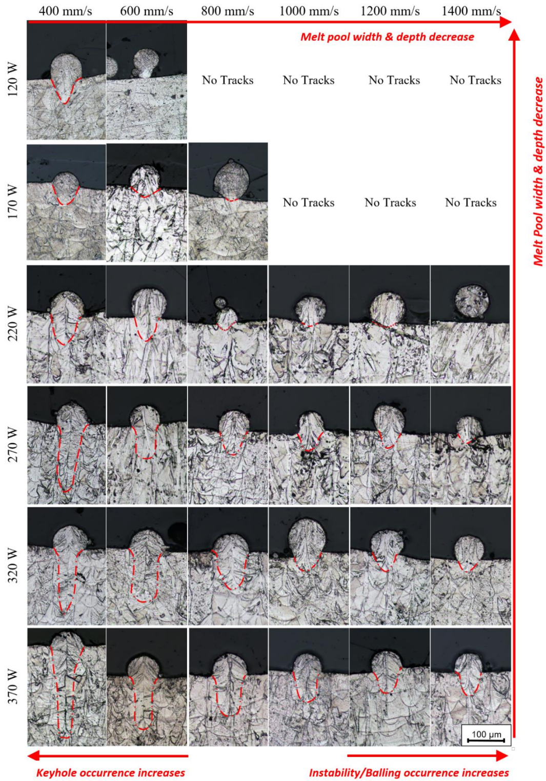
Figure 3-5 Cross-sectional view of etched single tracks melt pools
