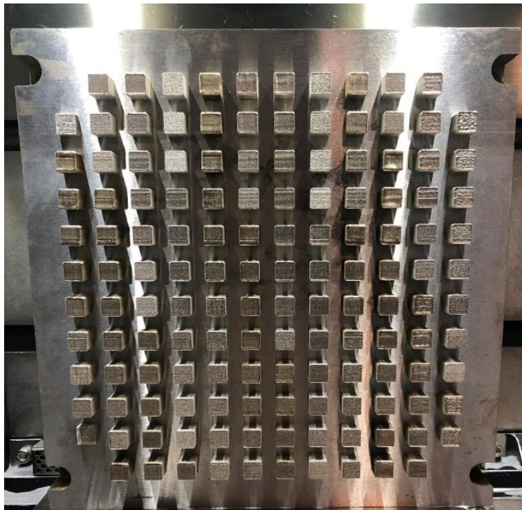
Figure 3-1 Inconel 718 cube coupons before separation from the build plate
