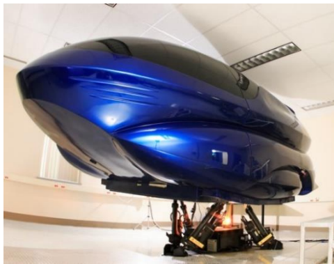
Figure 1. Motion platform and simulator system used for this study
