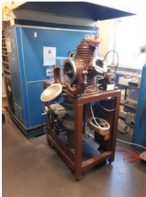
Figure 2-11 A general view of the setup used to calibrate the pyrometer.
