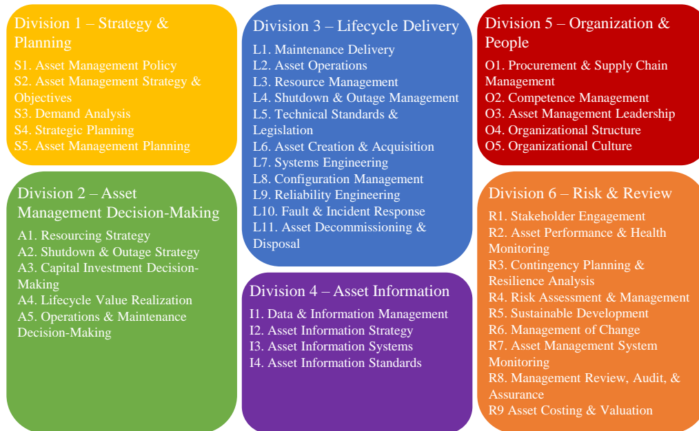
Figure 1-2. 39 AM subject areas illustrating the extent of AM activities within an AM system.
