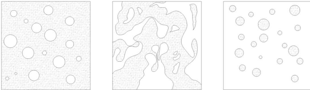
Figure 2.2. Morphological development of the dispersed phase and continuous matrix in binary low-affinity immiscible polymer blends.
