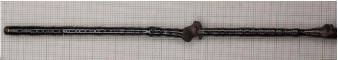
FIGURE 4.1: A continuous growth of Nd-LSCO  $x=0.17$ . The growth lasted for more than 250 hours. The crystal is about 13cm long.
