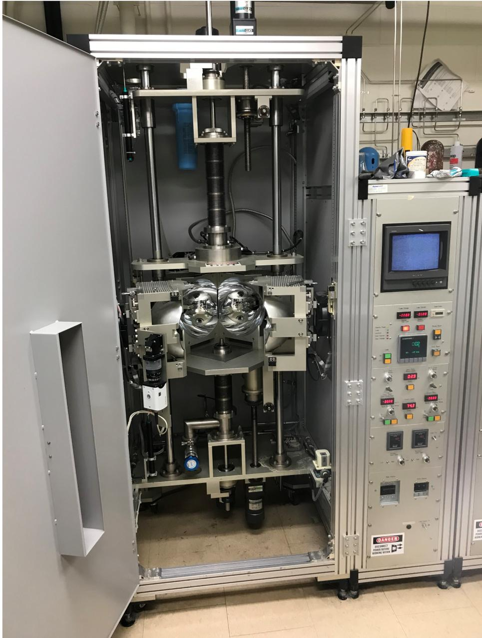
FIGURE 3.4: A photo taken at the Crystal System furnace at McMaster University's crystal growth lab.
