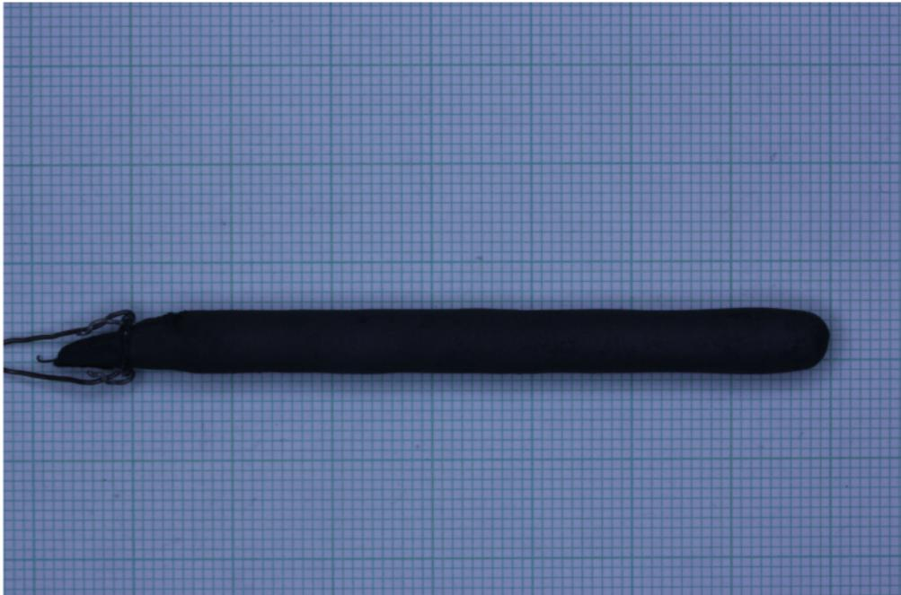
FIGURE 3.2: The feed rod of  $x=0.24$  sample. Photo taken after final annealing in flowing oxygen. The rod is about 7cm long and weighs 14.6 grams. Rod of this size can sustain two growths spanning over a time frame of two weeks.
