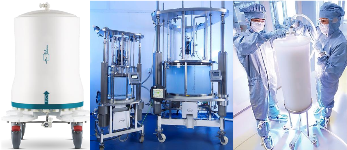
Fig. 1.12. Schematic of large-scale commercially available chromatography platforms; a) 8 L monolithic column; reprinted from BIA Separation ( www.biaseparations.com ); b) Resolute Linear chromatography (Pall) with 350mm-2000mm internal diameter; reprinted from Pall Biotech ( biotech.pall.com ); Copyright Pall Corporation; c) Membrane adsorber 54 ; Copyright Sartorius Stedim Biotech.
