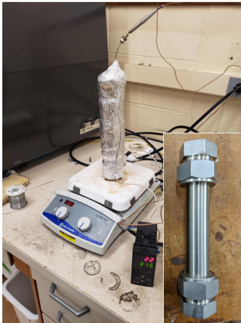
Figure 4.1: Experimental setup for the glycothermal reaction.
