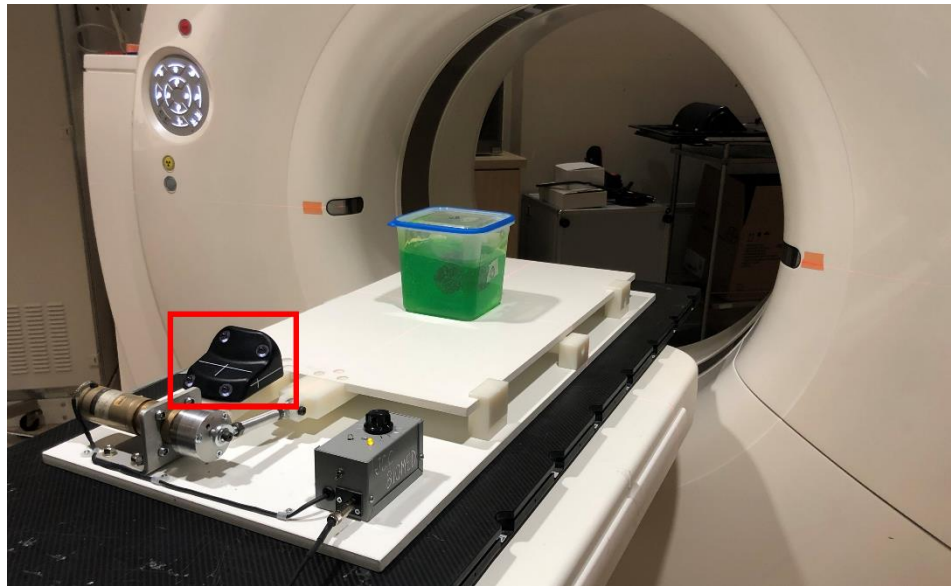
Figure 2.10 4DCT setup for imaging of irregular lesion. Note the device highlighted by the red square is the reflective block of the Varian Real-Time Position Management Respiratory Gating System. This device tracked the oscillation of the moving platform for the temporal component of 4DCT.
