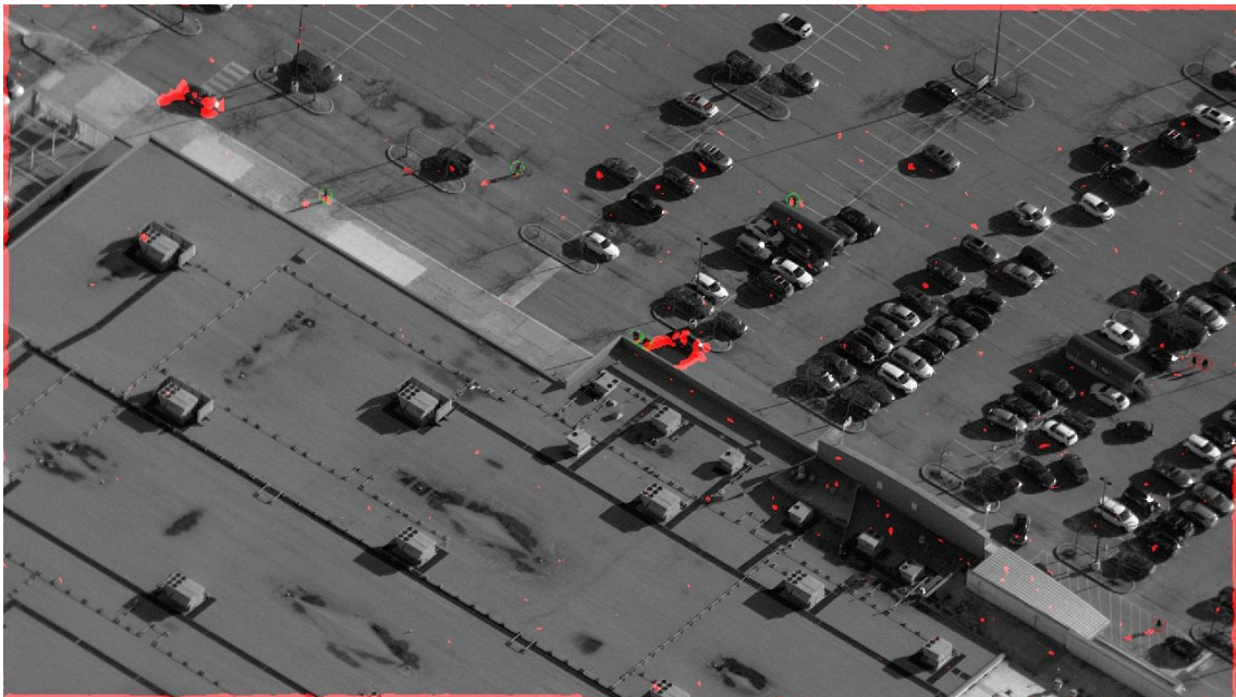
Figure 4.8: A visual representation of the optical flow detector. The detections identified by the algorithm are highlighted in red. The location of all accurately detected dismounts is marked with a green circle.
