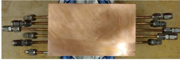
Figure 3-6 The soldered copper Oscillating Heat Pipe with the Swagelok fittings.
