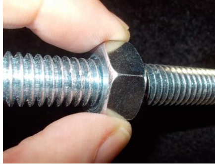
Figure 6.4-2. A simple nut-screw “experiment” to explain the movement of the packed solid bed in an extruder.
