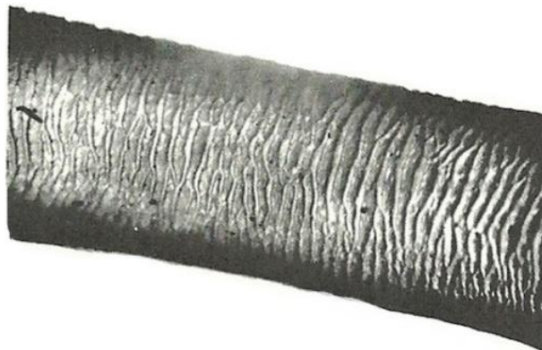
Figure 4.2-1. Typical sharkskin on an extrudate of about a 2 mm, exaggerated due to the enlargement. Note the formation of ridges perpendicular to flow direction. Adapted from Dennison (1967).
