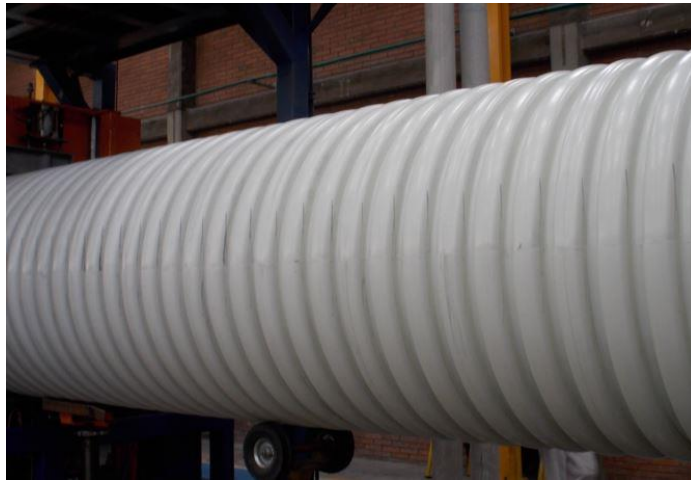
Figure 10.4-1. PVC 48 inch (1219 mm) pipe produced on Corma ( www.corma.com ) equipment.
