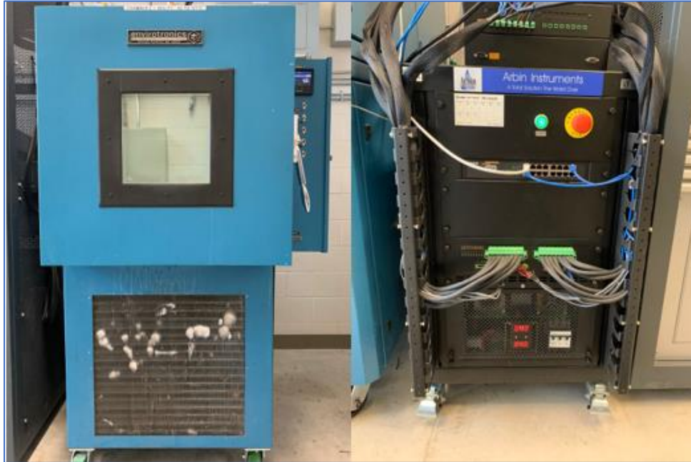
Figure 4.2: Environmental Chamber (left) and battery tester (right) utilized in the test.
