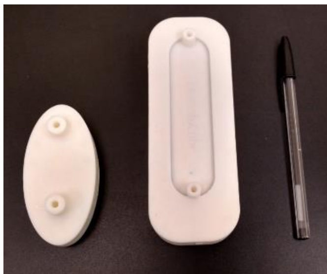
Figure A3. LFMC devices containing 1 mL (left) and 10 mL (right) of the Sartobind Q membrane.
