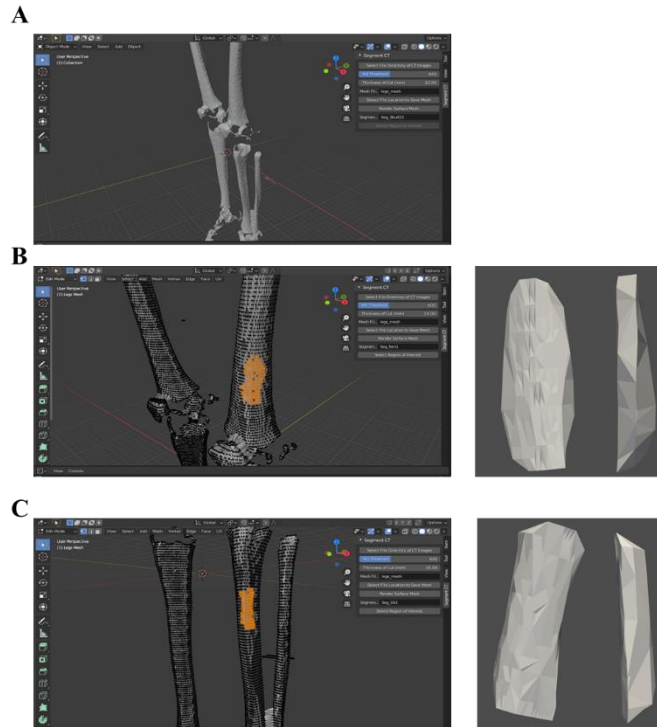
Figure 3. 51: Blender interface for a set of CT images of the lower limbs, A. mesh created by ‘Render Surface Mesh’, B. user selection and resulting STL (frontal and side view) for femur selection, and C. user selection and resulting STL (frontal and side view) for tibia selection. Both B. and C. used a thickness of the cut of 10.0 mm. Smoothing of the shape defined by the user occurred and the curvature of the inner and outer surface appeared to be maintained.
