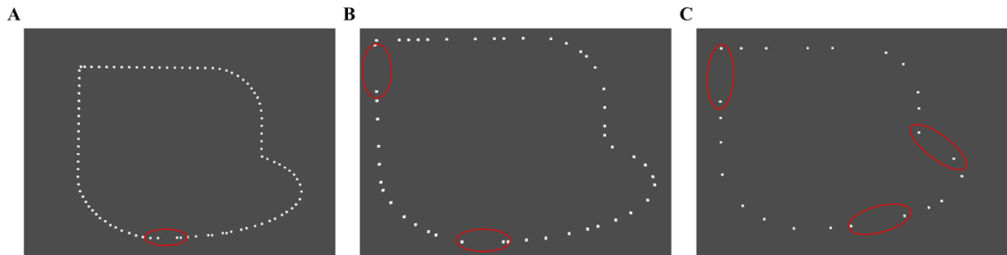
Figure 3. 38: Pseudo-uniform sampling with A. 9.94% (194 points), B. 4.92% (96 points), and C. 2.46% (48 points). Gaps created during the sampling algorithm are highlighted by red ovals but overall the shape was maintained.
