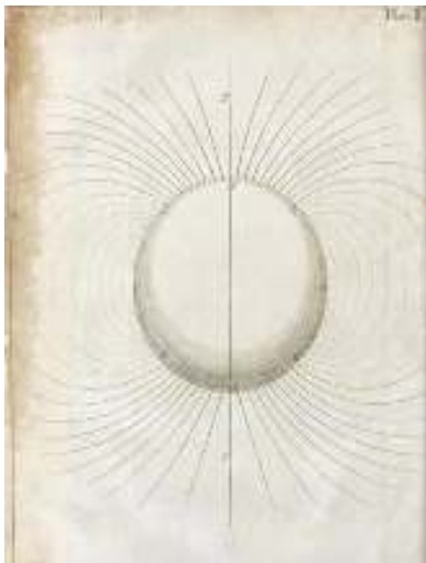
Figure 2.10 Diagram of Edmund Halley's experiment studying the placement of iron filings around a magnet where A and B represent the poles of Earth.
