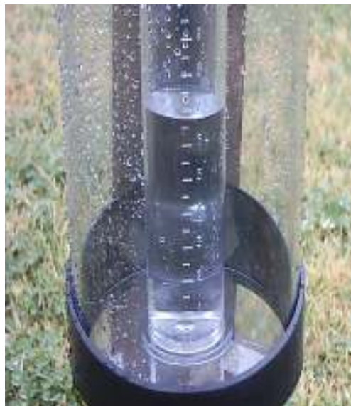
Figure 2.22 A modern rain gauge placed in the field and measuring over 6.5mm of rain. At the top of the gauge is a funnel (not pictured) that directs water inside the measurement cylinder. The funnel is 10 times the cross-sectional area of the cylinder. The gauge is therefore calibrated so that 1/10 of an inch of rain in the funnel corresponds to 1 inch of rain in the tube and 1 inch of rainfall.
