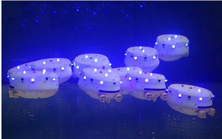
Figure 1.8: NLOS broadcast communication system using 12-LEDs transmitter (the image reproduced from [65])
